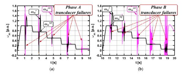
**Figure 10.** Measured, real, and estimated induction motor speed during the neural network training process (for phase A transducer failures (**a**) and for phase B transducer failures (**b**)).
