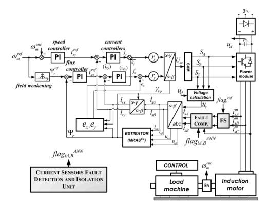
**Figure 8.** Scheme of the Direct Field Oriented Control (DFOC) structure with current sensor fault detection algorithm.
