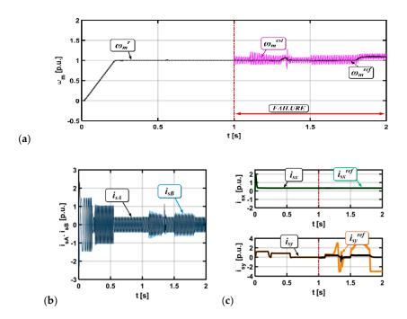
**Figure 6.** Results for the drive system with a broken current sensor in phase A (gain error), (rotor speed (a), stator current (b), stator current components x, y (c)).
