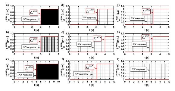
**Figure 15.** Experimental results of the transients of the output signals from a neural detector during failures of the phase A current transducer:  $\omega_m = \omega_{mN}$ ,  $m_o = m_{oN}$  (**a**,**d**,**g**),  $\omega_m = 0.05\omega_{mN}$  (**b**,**e**,**h**),  $\omega_m = \omega_{mN}$ ,  $m_o = m_{oN}$  reverse operation (**c**,**f**,**i**)—total failure of the sensor (**a**,**b**,**c**), white noise (**b**,**c**,**d**) and gain change (**g**,**h**,**i**).
