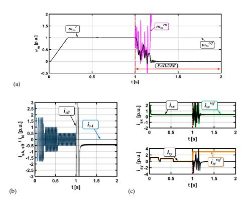
**Figure 4.** Results for the drive system with a broken current sensor in phase A (lack of signal), (rotor speed (**a**), stator current (**b**), stator current components x,y (**c**)),  $i_A' = 0$ .
