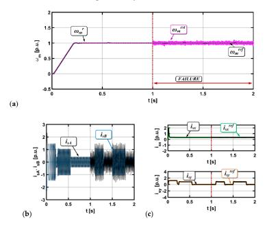
**Figure 7.** Results for the drive system with a broken current sensor in phase A (white noise), (rotor speed (**a**), stator current (**b**), stator current components x,y (**c**)).
