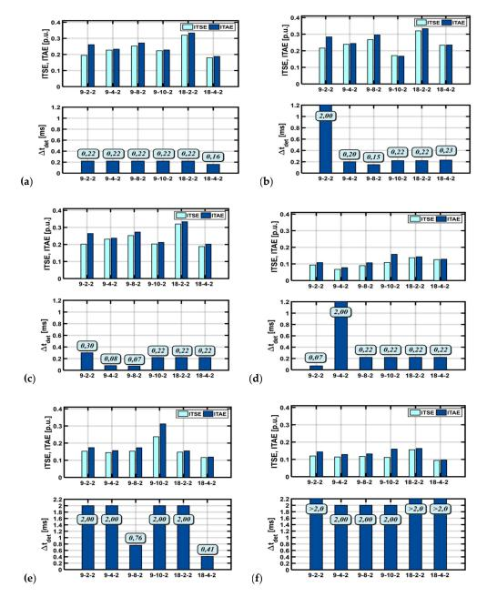
**Figure 11.** Bar charts with the values of ITSE and ITAE integral quality indicators and fault detection times for different NN learning cycles: (**a**,**d**) operation of the drive with a rated speed value, (**b**,**e**) rated speed and load torque values, (**c**, **f**) low speed value failure detection of the current transducer phase A (**a**, **b**, **c**) and phase B (**d**, **e**, **f**), simulation results.
