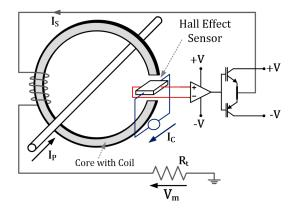
Figure 2. Current sensor scheme based on the Hall effect.
