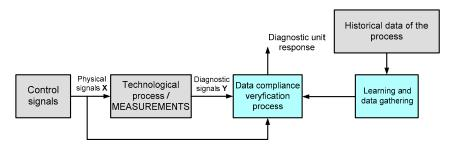
Figure 1. Data analysis based diagnostic system—general diagram.
