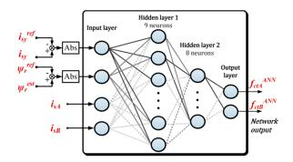
Figure 12. Schematic diagram of designed NN-based detector.
