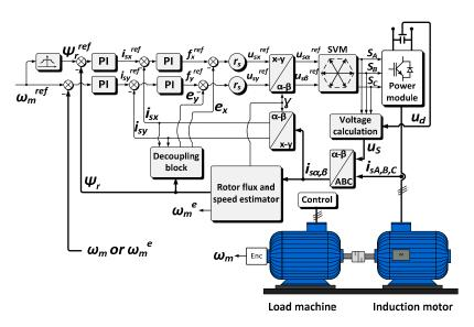
Figure 3. General scheme of the Direct Rotor Field Oriented Control (DRFOC).
