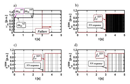
**Figure 14.** Experimental results of (**a**) measured, real, and estimated rotor speed during: (**b**) total failure of the phase B current transducer, (**c**) white noise, and (**d**) gain change,  $\omega_m = 1.25\omega_{mN}$
