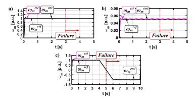
**Figure 13.** Measured, real, and estimated rotor speed during total failure of the phase A current transducer: (a)  $\omega_m = \omega_{mN}$ ,  $m_o = m_{oN}$ , (b)  $\omega_m = 0.05\omega_{mN}$ , and (c)  $\omega_m = \pm \omega_{mN}$ ,  $m_o = m_{oN}$  reverse operation—experimental results.
