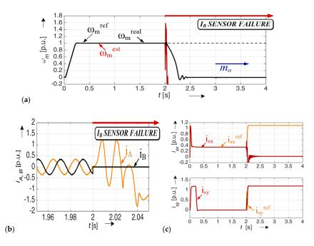
**Figure 5.** Results for the drive system with a broken current sensor in phase B (lack of signal), (rotor speed (**a**), stator current (**b**), stator current components x,y (**c**)),  $i_B' = 0$ .
