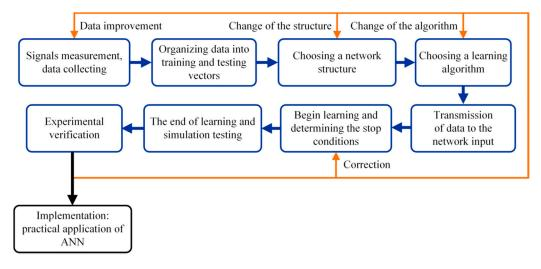
Figure 9. Neural network design cycle [17].
