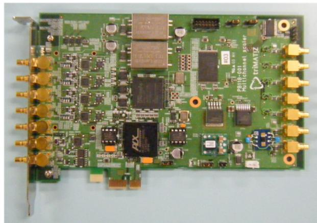
Figure 7. Photon counting device (Trimatiz Co. Ltd, “Photon Tracker”).
