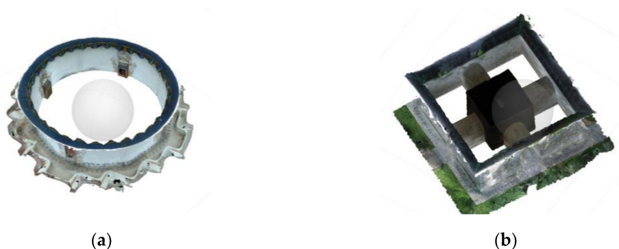
Figure 6. Textured mesh model with recovered frame positions of the two datasets. (a) B_{30} of the Stupa; and (b) B_{30} of the Pavilion.
