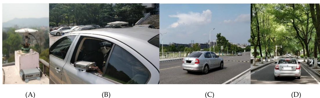
Figure 3. Equipment setup and navigation test environment: (A) Base station; (B) Rover station; (C) Open-sky road; (D) Signal blocked road.
