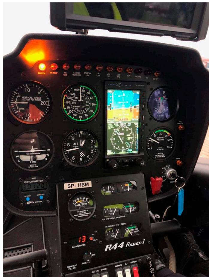
**Figure 2.** Avionics of the Robinson R44 Raven helicopter.
