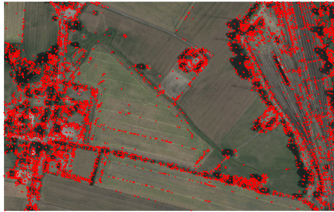
Figure 6. Orthophotomap with marked keypoints processed using the ASIFT algorithm.
