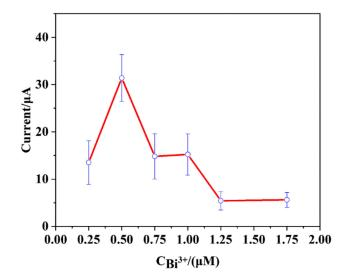
**Figure 9.** Effect of concentration of  $Bi^{3+}$  solution on the stripping peak current of 0.5 µmol/L of Cd<sup>2+</sup> at Bi/CMC-GCE in NaAc/HAc buffer solution (0.10 M, pH 4.5). The investigated concentration of  $Bi^{3+}$  solution were 0.25, 0.50, 0.75, 1.00, 1.25, 1.50, 1.75 µmol/L. CMC solution: 0.4 mg/mL; accumulation time 180 s; deposition potential: -1.2 V; scan rate: 50 mV·s<sup>-1</sup>.
