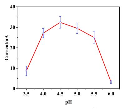
**Figure 5.** Effect of pH on the stripping peak current of 0.5  $\mu$ mol/L of Cd<sup>2+</sup> at Bi/CMC-GCE in 0.10 mol/L of NaAc/HAc buffer solution. The investigated pH values were 3.5, 4.0, 4.5, 5.0, 5.5, and 6.0. Deposition potential: -1.2 V; accumulation time: 150 s; scan rate: 50 mV·s<sup>-1</sup>.
