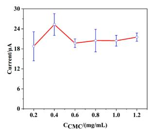
**Figure 8.** Effect of concentration of CMC on the stripping peak current of 0.5  $\mu$ mol/L of Cd<sup>2+</sup> at Bi/CMC-GCE in NaAc/HAc buffer solution (0.10 mol/L, pH 4.5). The investigated concentration of CMC were 0.2, 0.4, 0.6, 0.8, 1.0, and 1.2 mg/mL. Accumulation time 180 s; deposition potential: -1.2 V; scan rate: 50 mV·s<sup>-1</sup>.
