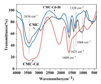
Figure 1. FT-IR spectra of sodium carboxymethyl cellulose (CMC) and its complexes CMC-Cd and CMC-Cd-Bi.
