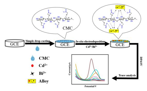
**Scheme 1.** Strategy for the construction of the new cadmium electrochemical sensor based on synergetic effects of both CMC and bismuth on the enrichment and detection of cadmium ions.
