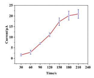
**Figure 6.** Effect of accumulation time on the stripping peak current of 0.5  $\mu$ mol/L of Cd<sup>2+</sup> at Bi/CMC-GCE in NaAc/HAc buffer solution (0.10 mol/L, pH 4.5). The investigated accumulation times were 30 s, 60 s, 90 s, 120 s, 150 s, 180 s, and 210 s. Deposition potential, -1.2 V; scan rate: 50 mV·s<sup>-1</sup>.
