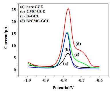
**Figure 4.** Differential pulse anodic stripping voltammograms for 0.5  $\mu$ mol/L of Cd<sup>2+</sup> in NaAc/HAc (0.10 mol/L, pH 4.5) buffer solution at the surface of bare GCE (**a**), CMC-GCE (**b**), Bi-GCE (**c**) and Bi/CMC-GCE (**d**). Deposition potential: -1.2 V; accumulation time 150 s; scan rate: 50 mV·s<sup>-1</sup>.
