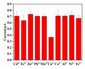
**Figure 11.** Interferences caused by co-existing cations (5  $\mu$ mol/L) on the stripping peak current of 0.2  $\mu$ mol/L Cd<sup>2+</sup>. All measurements were carried out under the optimized experimental conditions. CMC solution: 0.4 mg/mL; bismuth ion solution: 0.5  $\mu$ mol/L; pH 4.5; deposition potential: -1.2 V; accumulation time: 180 s; scan rate: 50 mV·s<sup>-1</sup>.
