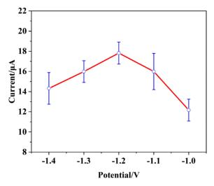
**Figure 7.** Effect of deposition potential on the stripping peak current of 0.5  $\mu$ mol/L of Cd<sup>2+</sup> at Bi/CMC-GCE in NaAc/HAc buffer solution (0.10 mol/L, pH 4.5). The investigated deposition potentials were –1.4 V, –1.3 V, –1.2 V, –1.1 V, and –1.0 V. Accumulation time 180 s; scan rate: 50 mV·s<sup>-1</sup>.
