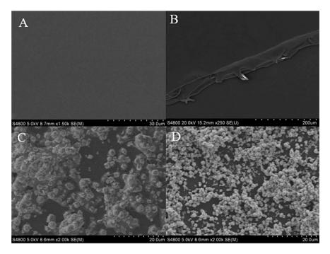
**Figure 2.** SEM images of the bare glassy carbon electrode (GCE) (**A**), CMC-GCE (**B**), bare GCE after electrodeposition of cadmium and bismuth (**C**), and CMC-GCE after electrodeposition of cadmium and bismuth (**D**).
