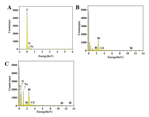
**Figure 3.** EDS spectra of CMC-GCE (**A**), bare GCE after electrodeposition of cadmium and bismuth (**B**), and CMC-GCE after electrodeposition of cadmium and bismuth (**C**).
