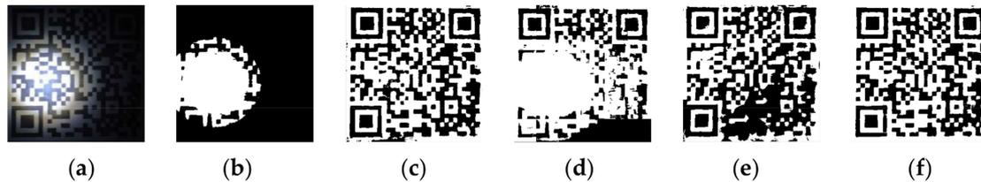
**Figure 12.** The original image and experimental results from different algorithms: (a) Original image; (b) Otsu's algorithm; (c) Niblack's algorithm; (d) Yao's algorithm; (e) Di's algorithm; (f) Proposed method.
