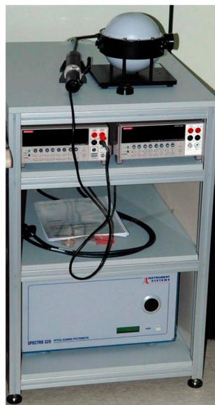
**Figure 4.** Configuration of the spectrometer system.
