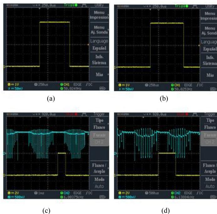
**Figure 12.** PWM signals generated by the Arduino Nano microcontroller: (a) PWM signal of average speed; (b) PWM signal of maximum speed; (c) PWM signal of minimum speed and output signal of ESC30A controller; and (d) PWM signal of maximum speed and output signal of ESC30A controller.
