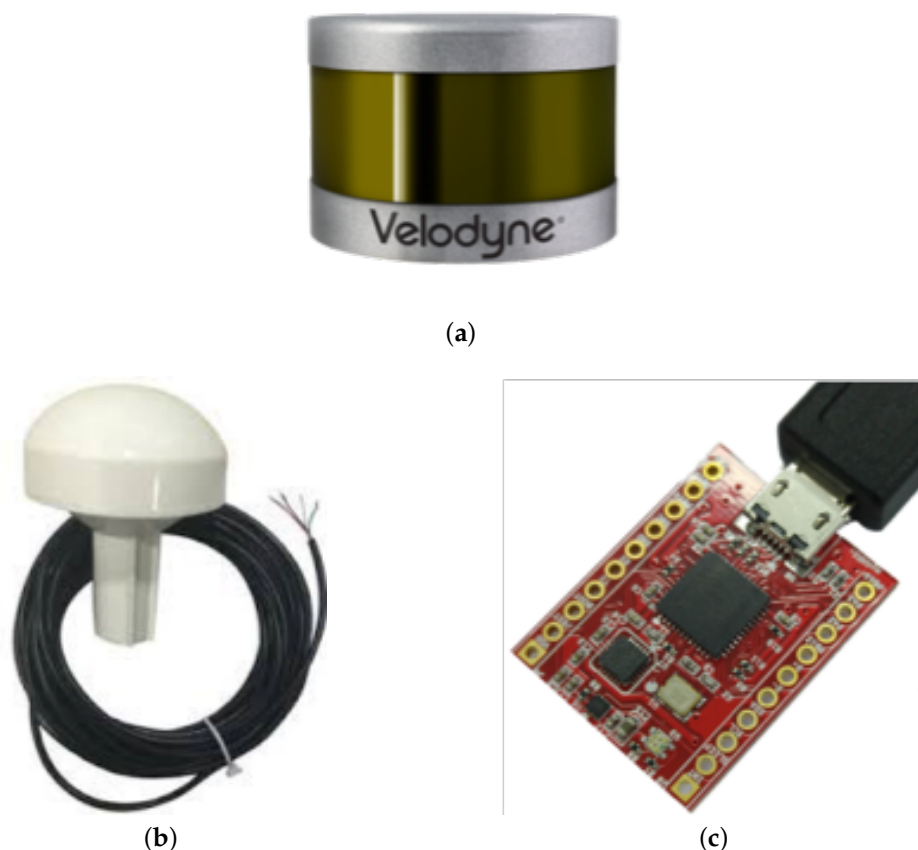
Figure 1. VLP-16 LiDAR (a), GPS receiver (b), and low cost attitude heading and reference system (AHRS) (c) used in the portable 3D data acquisition system.
