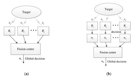
Figure 9. Topology structure diagram of fusion detection: (a) Measurement fusion; (b) Decision fusion.
