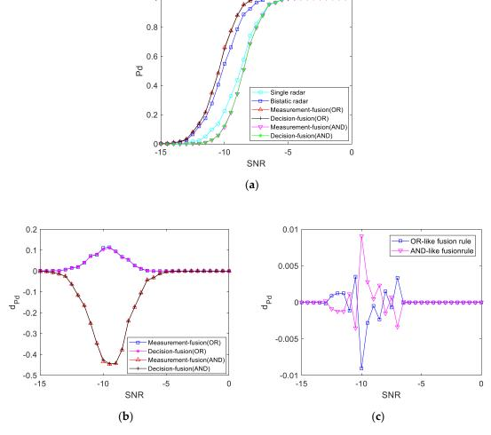
**Figure 13.** Bistatic radar echo power is greater than single radar echo power: (a) Detection performance curve; (b) Difference value of the detection performance curve with the bistatic radar; (c) Difference value of the fusion detection performance curve.
