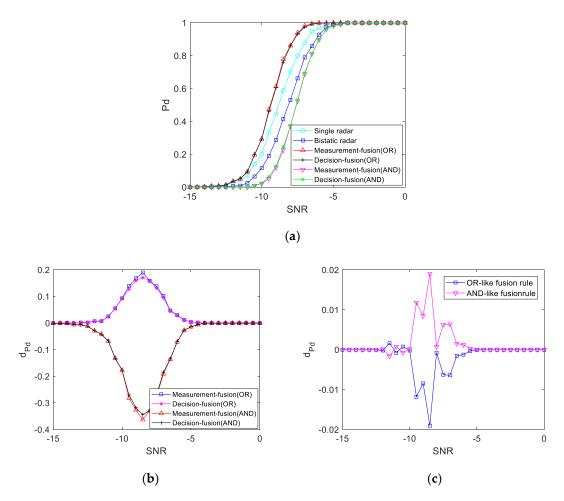
**Figure 15.** Single radar echo power is greater than bistatic radar echo power: (a) Detection performance curve; (b) Difference value of the detection performance curve with a single radar; (c) Difference value of the fusion detection performance curve.
