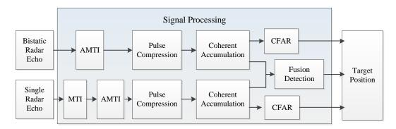
Figure 3. Block diagram of the radar echo processing for the cooperative detection system.
