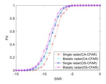
Figure 12. Detection performance curve of the CFAR algorithm.
