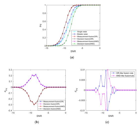
**Figure 14.** Single and double base target echo signal power is the same: (a) Detection performance curve; (b) Difference value of the detection performance curve with a bistatic radar; (c) Difference value of the fusion detection performance curve.
