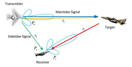
Figure 1. Scene schematic diagram of cooperative irradiation.
