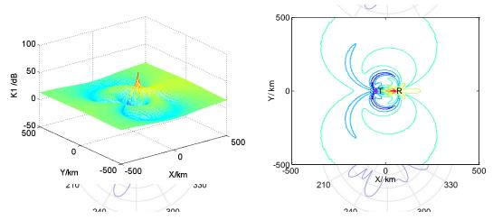
**Figure 6.** The value of the distribution of  $K_1$ : (a) Three-dimensional distribution of  $K_1$ ; (b) The isogram of the distribution of  $K_1$ .
