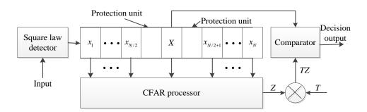
Figure 8. CFAR processor architecture.
