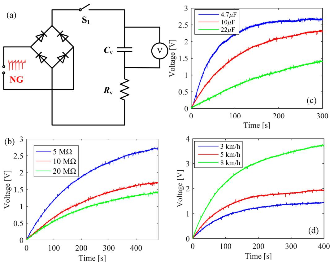
**Figure 4.** Charging characteristics test of the insole. (a) Circuit diagram. (b) Charging curve with different values of  $R_v$  and  $C_v = 22 \mu\text{F}$ . (c) Charging curve with different values of  $C_v$  and  $R_v = 10 \text{ M}\Omega$ . (d) Charging curve with different motion speed when  $R_v = 10 \text{ M}\Omega$  and  $C_v = 10 \mu\text{F}$ .
