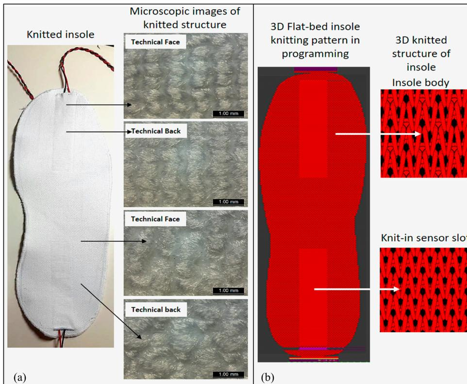
Figure 2. (a) Prototype and (b) structure of the self-powered smart insole.
