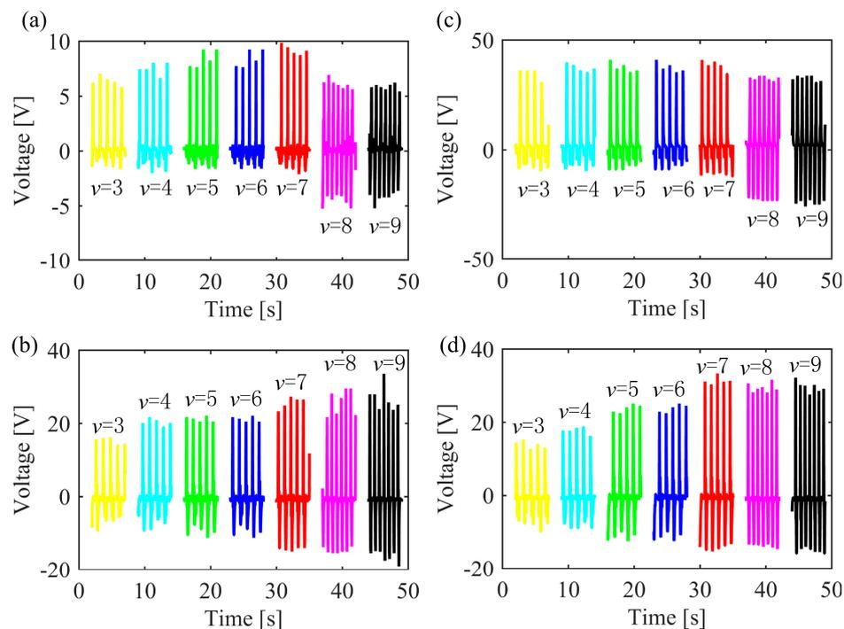
**Figure 3.** Voltage response of the insole under different motion speed from 3 km/h to 9 km/h: (a) left forefoot; (b) left hindfoot; (c) right forefoot; (d) right hindfoot.
