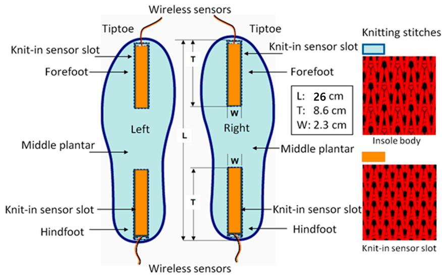
Figure 1. Schematic diagram of the self-powered smart insole.
