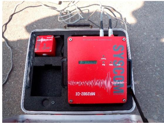
Figure 3. MR2002-CE type signal recorder.
