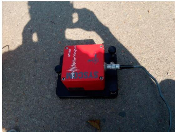
Figure 4. MS2003 speedometer.
