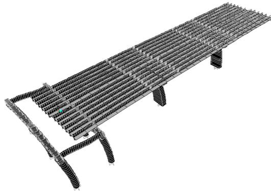
Figure 20. Bridge model after completion of P9 jacking (1).
