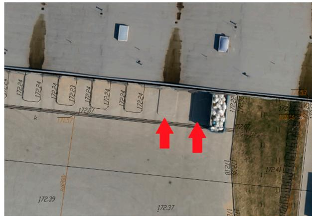
**Figure 12.** Visualization of the deficiencies on the vector base map using orthomosaic in AutoCAD.
