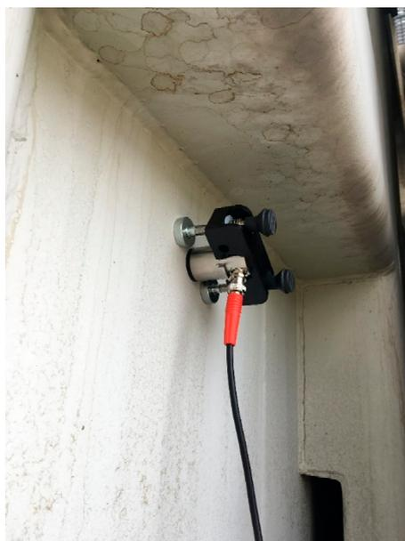
**Figure 1.** General view of the acoustic emission (AE) sensor during measurements on a 150 MVA power transformer.
