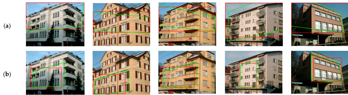
Figure 11. The extracted low-rank texture regions and the results processed by the TILT algorithm. (a) The results obtained with the method proposed in [34]. (b) The results obtained using the proposed low-rank texture region detection algorithm. The red lines denote the input to the TILT algorithm, and the green lines denote the returned deformed textures.
