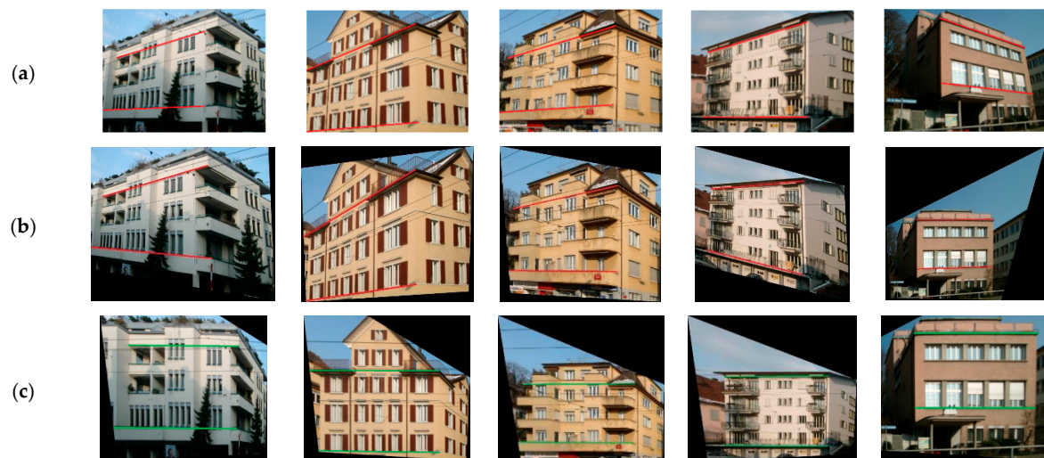
Figure 12. Comparative results of the image rectification. The lines marked in the images are the parallel lines in the real scenes. (a) Original; (b) Zhang et al. [34]; (c) Proposed.
