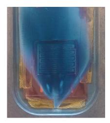
**Figure 1.** View of the steel hot wall reactor, opened after the aerosol-assisted chemical vapor deposition (AA-CVD) process. Kapton mask (brown), Ag stenciled tracks, and grown WO<sub>3</sub> (blue) can be observed.
