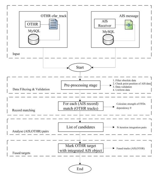
**Figure 1.** Algorithm for the fusion of automatic identification system (AIS) data and over-the-horizon radar (OTHR) tracks.
