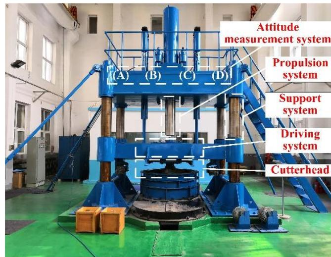
**Figure 10.** Experimental platform of attitude measurement system.
