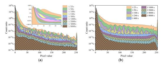
**Figure 3.** Distribution of the count fraction of pixels at a dose rate of 51.61 Gy/h and (a) a gain of 6 dB and (b) a gain of 42 dB in frames captured at using integration times ranging from 1/8000 to 1/25 s.
