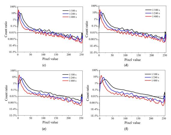
**Figure 5.** Distribution of the count fractions of pixels at a gain of 6 dB for six different dose rates in frames captured at integration times of 1/100, 1/240, and 1/480 s: (a) 64.48, (b) 95.00, (c) 119.5, (d) 153.41, (e) 200.32, and (f) 265.22 Gy/h.
