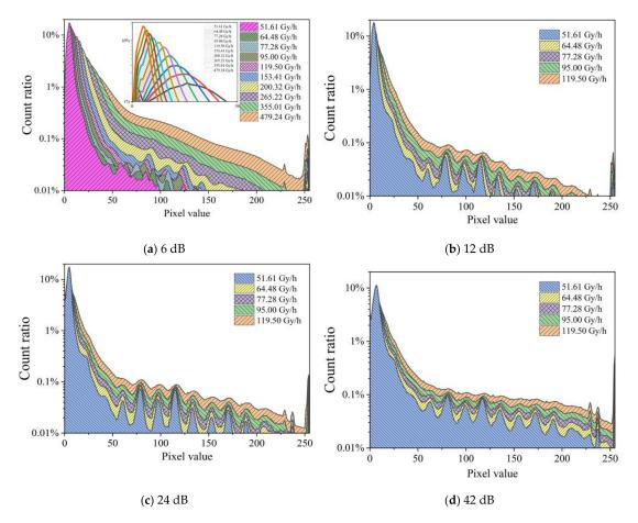
**Figure 9.** Distribution of the count fraction of pixels at an integration time of 1/100 s for four values of the gain captured at dose rates ranging from 51.61 to 119.50 Gy/h (from **b** to **d**), and from 51.61 to 479.24 Gy/h (**a**).
