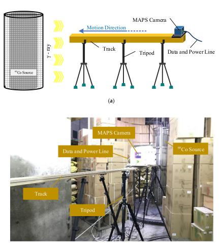
**Figure 2.** Experimental setup: (a) Schematic view of the experimental system and (b) picture of the experimental setup.
