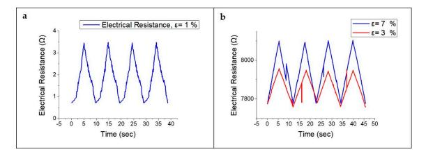
**Figure 9.** Response of LIG strain sensor under stretch/release cycle of (a)  $\varepsilon = 1\%$ ; (b)  $\varepsilon = 3\%$  and 7%.
