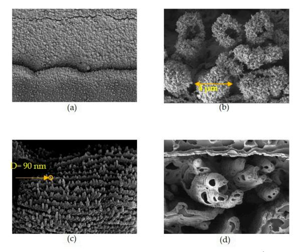
**Figure 4.** Laser fluence-dependent SEM images of LIG pattern; laser fluence of (**a**) 5.6 J/cm<sup>2</sup>; (**b**) 5.9 J/cm<sup>2</sup>; (**c**) 6.4 J/cm<sup>2</sup>; (**d**) 7.4 J/cm<sup>2</sup>.
