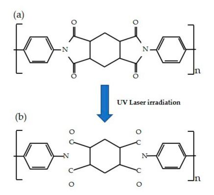
**Figure 2.** Principle of laser-induced graphene (LIG). (**a**) Structure of polyimide film; (**b**) Structural change of polyimide film after laser irradiation.
