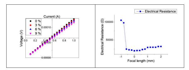
**Figure 10.** (**a**) Electrical response of LIG strain sensor; (**b**) Change of initial electrical resistance according to focal length.
