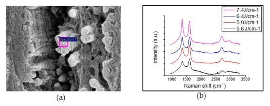
**Figure 5.** The graphene-like flake structure of the LIG pattern; (**a**) SEM image of the graphene-like flake structure of LIG; (**b**) Raman spectra of the LIG pattern irradiated laser with different laser fluences.
