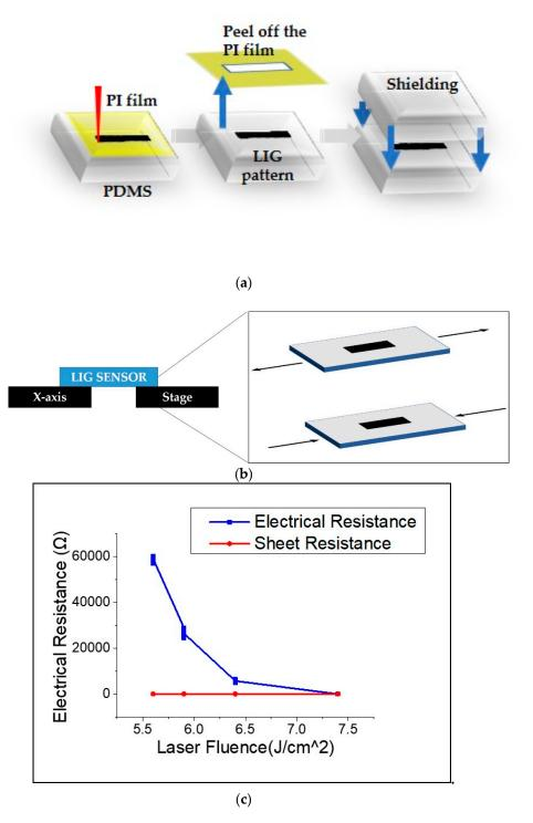
**Figure 3.** Fabrication of LIG sensor: (**a**) process of fabricating the LIG strain sensor, (**b**) strain generation by bending, and (**c**) changes in electrical characteristics according to laser fluence.
