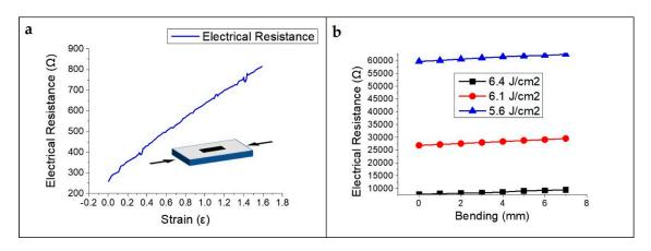
**Figure 7.** Change in electrical resistance corresponding to strain with each laser fluence: (**a**) 7.4 J/cm<sup>2</sup>; (**b**) 5.6 to 6.4 J/cm<sup>2</sup>.
