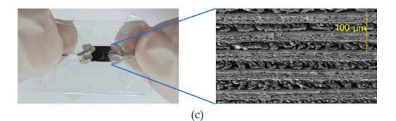
**Figure 6.** Photographs of the strain sensor under (**a**) twisting and (**b**) bending; (**c**) SEM image of carbonized pattern embedded on polydimethylsiloxane (PDMS).
