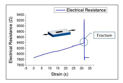
Figure 8. Change in electrical resistance corresponding to strain and fracture.
