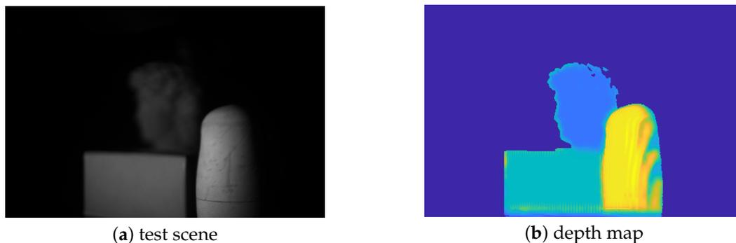
**Figure 7.** Photograph of the test scene and the global coarse depth map. (a) Test scene; (b) depth map.
