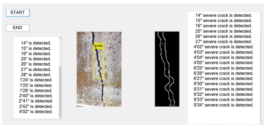
Figure 3. Operation interface for crack detection of retaining wall.
