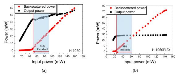
Figure 4. SBS threshold power measurements for (a) HI1060 fiber and (b) HI1060FLEX fiber.
