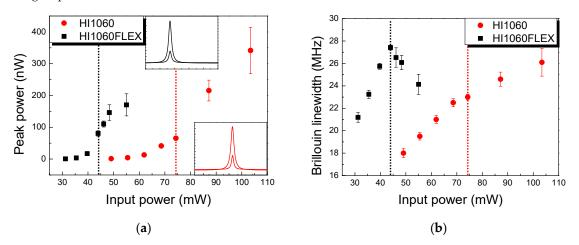
**Figure 3.** Variation of (**a**) SBS peak power and (**b**) linewidth  $\Delta v_B$  as a function of the input laser power at  $\lambda = 1064$ nm in the room temperature for HI1060 and HI1060FLEX fiber with the length of 500 m.
