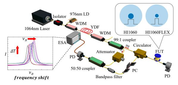
**Figure 1.** Schematic diagram of the all-fiber optical heterodyne SBS measurement set-up for passive 1060 nm single mode fibers (SMFs) (Corning HI1060, HI1060Flex) (YDF: Yb-doped fiber; WDM: wavelength division multiplexer; LD: laser diode; PD: photodetector; PC: polarization controller; FUT: fiber under test; ESA: electric spectrum analyzer).
