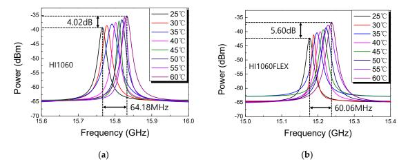
**Figure 5.** Measurements of Brillouin spectra as a function of temperature. (a) HI1060, (b) HI1060FLEX. Here the input signal power was 55 mW at  $\lambda$  = 1064nm and the fiber lengths were 500m.
