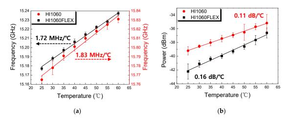
**Figure 6.** Temperature-dependent Brillouin peak parameters for HI1060 and HI1060FLEX fibers with the incident power of 55 mW. (**a**) The Brillouin frequency  $v_B$  and (**b**) the peak power. The fiber lengths were 500 m.
