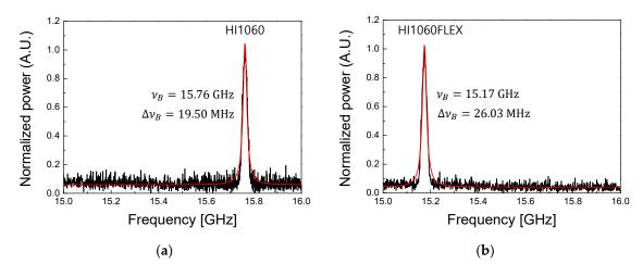
**Figure 2.** Stimulated Brillouin scattering (SBS) spectra measured by the experimental setup in Figure 1. The two 1060 nm SMFs, (**a**) HI1060 and (**b**) HI1060FLEX, had the equal length of 500 m and the measurements were made at the room temperature, the red curves are the Lorentzian fitting. Here the signal power incident to FUT was about 55 mW at  $\lambda = 1064$  nm.
