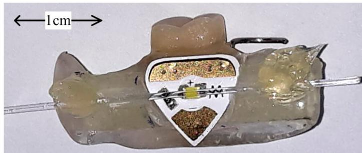
**Figure 4.** Practical realization of the point intra-oral sensor laboratory proof of concept, which has the LED source and the optical fiber from the sensor structure integrated into a lateral mouthguard.
