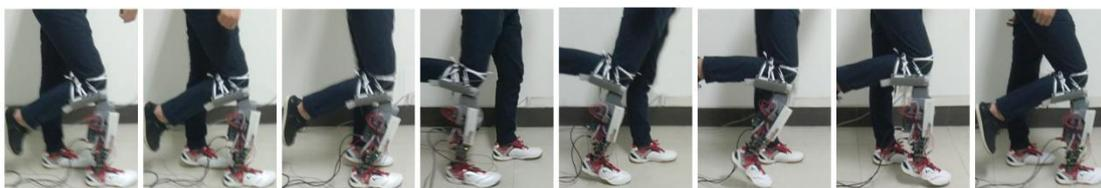
Figure 18. One gait cycle of the experimental level-ground walking.
