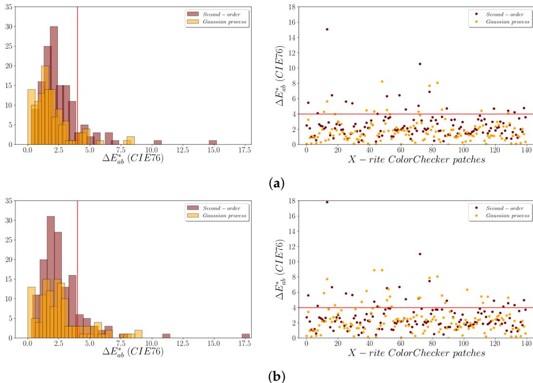
**Figure 4.** Sigma SD15  $\Delta E_{ab}^*$  values for the X-Rite patches: (a)  $\Delta E_{ab}^*$ ; (b) LOOCV  $\Delta E_{ab}^*$ .
