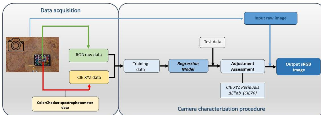
Figure 1. Schematic diagram designed for the camera characterization.
