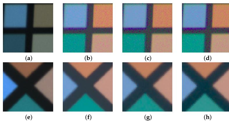
**Figure 7.** Noise comparative detail sRGB images after characterization: (a–d) Sigma SD15; (e–h) Fujifilm IS PRO; (a,e) Original raw images; (b,f) Gaussian process; (c,g) Second-order polynomial model; (d,h) Linear model.
