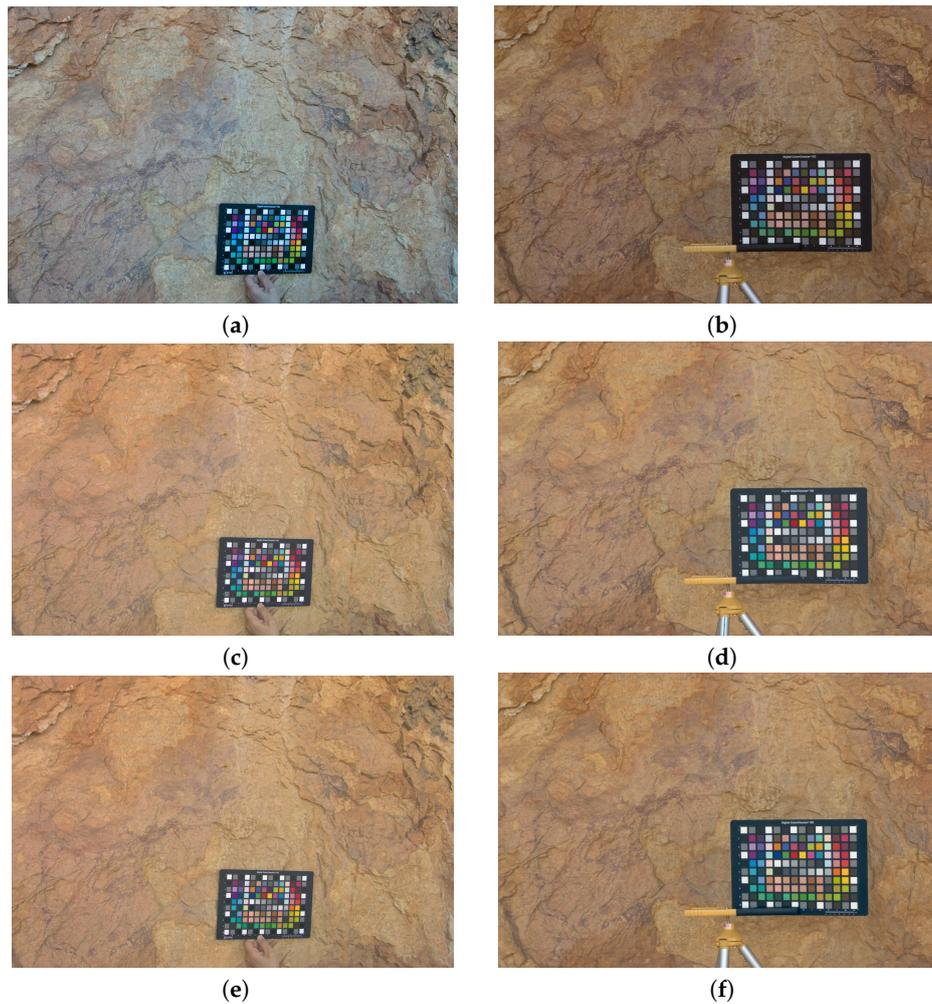
**Figure 8.** Original and output sRGB characterized images: (a,c,e) Sigma SD15; (b,d,f) Fujifilm IS PRO; (a,b) Original; (c,d) GP; (e,f) Second-order polynomial model.
