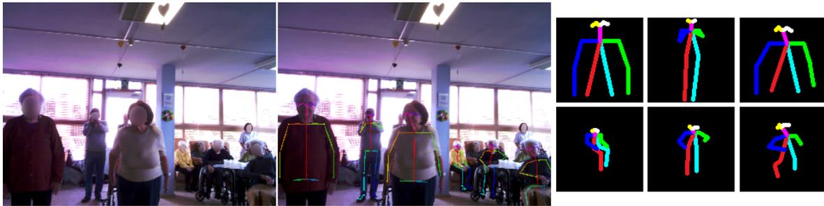
**Figure 2.** Human representation in terms of limbs by using Openpose: (left) Original image taken by the Pepper robot; (middle) Openpose output as body keypoint coordinates; (right) The human skeleton colour-coded to properly distinguish each limb (one per person).
