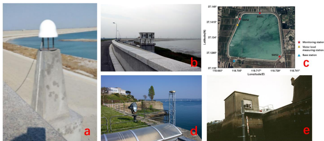
Figure 3. (a) Deformation monitoring station with radome; (b) Water level station at Shuangwangcheng Reservoir; (c) Dam monitoring stations and an overview of the reservoir; (d) The BRST station at the Atlantic coast of France; (e) Tide station near BRST station.
