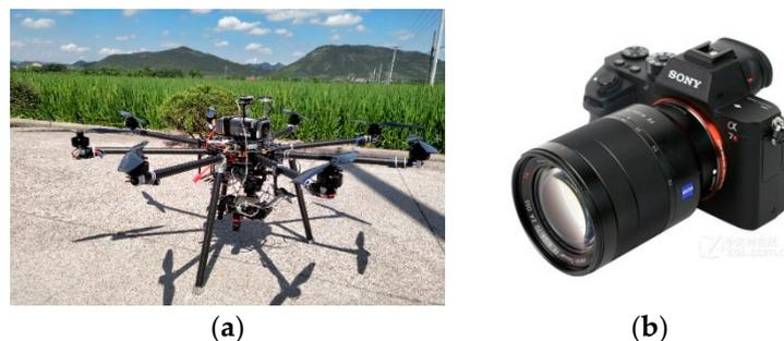
**Figure 1.** Sensing platform and photography equipment. (a) Eight-rotor UAV. (b) Sony A7RII full-range micro-single camera.
