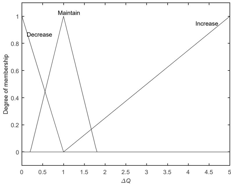
Figure 12. Member function of output  $\Delta Q$ .
