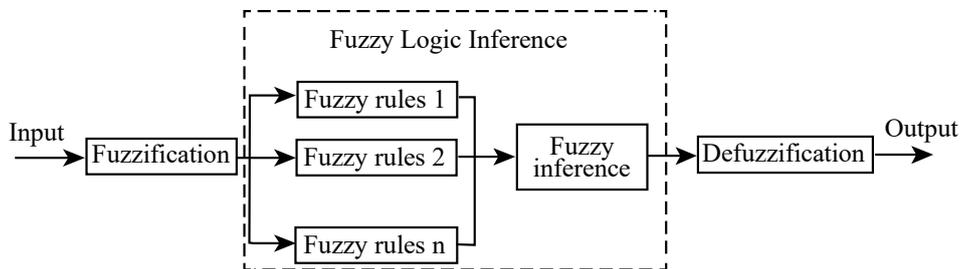
Figure 9. Structure of fuzzy inference system (FIS).
