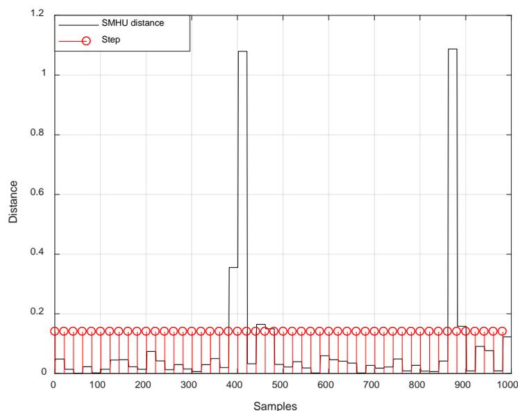
Figure 7. Corresponding distance change at each foot step by ultrasonic sensor.
