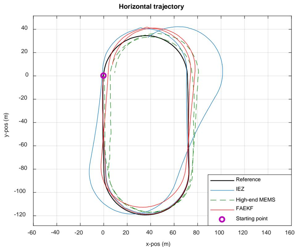
**Figure 14.** Estimated horizontal trajectories of PNS with different methods.
