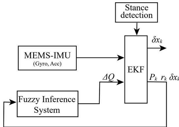
Figure 8. Block diagram of fuzzy adaptive EKF (FAEKF) for PNS.
