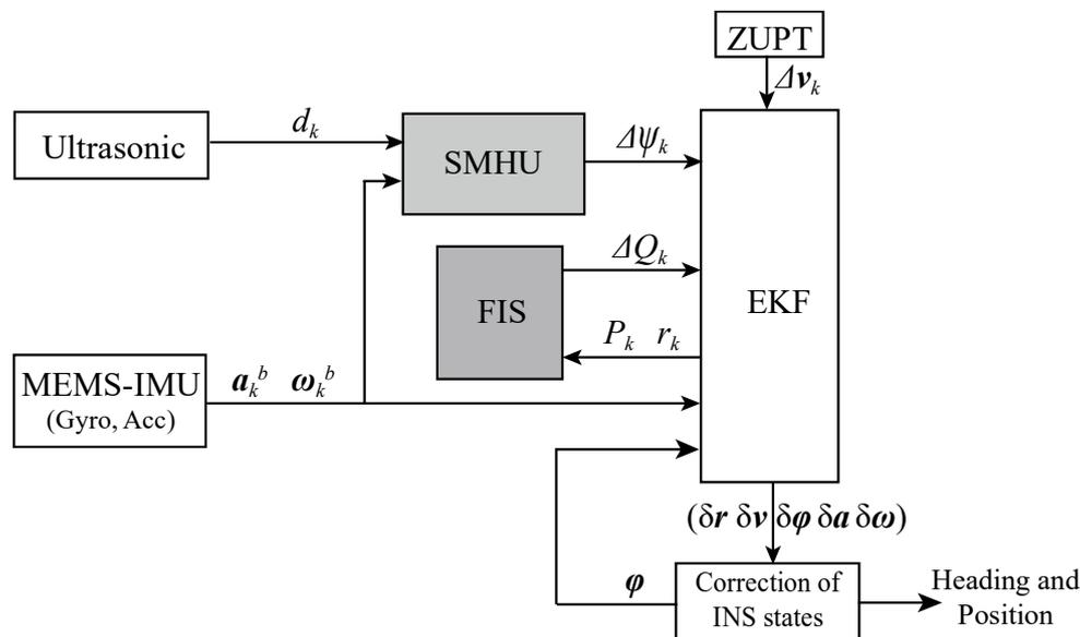
Figure 1. Structure of proposed positioning system.
