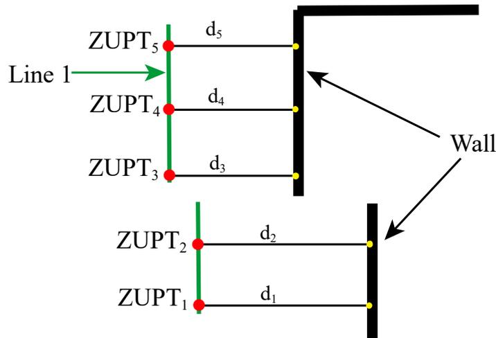
Figure 4. Straight line detection and formation by ultrasonic ranging and MEMS-IMU.
