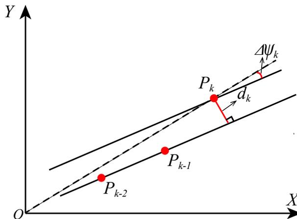
Figure 5. Calculation of heading drift due to gyro bias.
