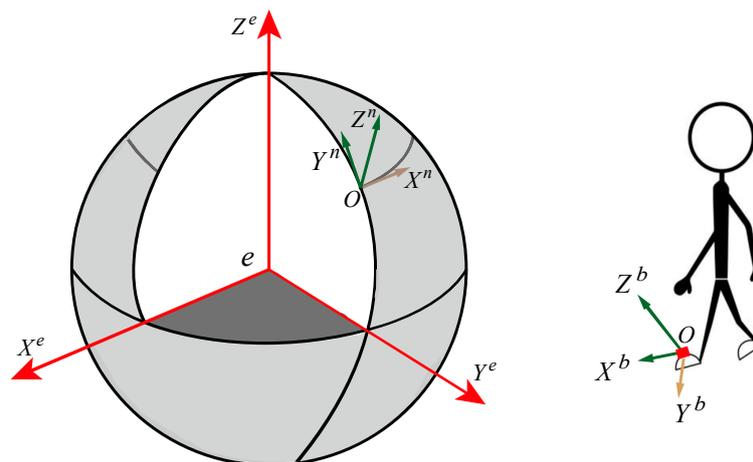
Figure 2. The reference frames involved in the algorithm.
