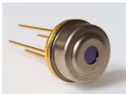
Figure 5. Photography of the TO-5 metal can package which the thermopile is sealed and die-bonding inside.
