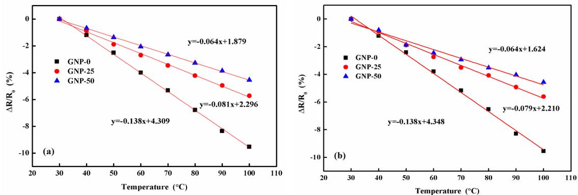
**Figure 11.** Normalized relative resistance change of the hybrid films varied with temperature. (a) Atmosphere environment; (b) Vacuum oven.
