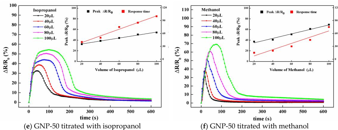
**Figure 15.** Resistance changes of the hybrid films titrated with different amounts of isopropanol and methanol.
