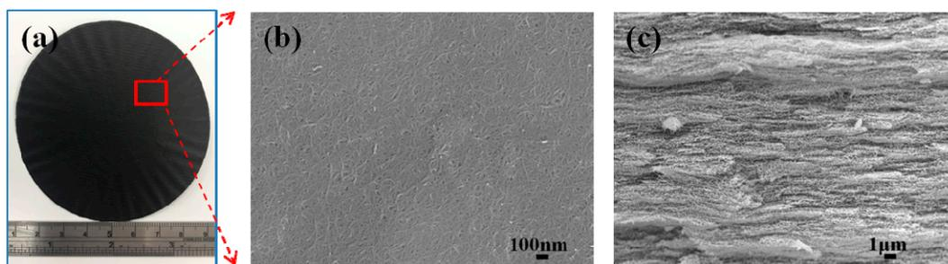
**Figure 4.** GNP-0 film with 0 wt% graphene and 100 wt% MWCNT; (a) the prepared film, (b) surface morphology SEM image, and (c) cross-section SEM image.
