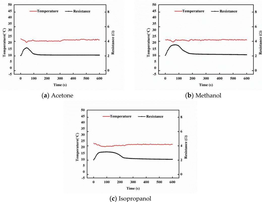
**Figure 16.** Temperature and resistance responses of the hybrid film GNP-50 titrated with 100  $\mu\text{L}$  of acetone, methanol, and isopropanol.
