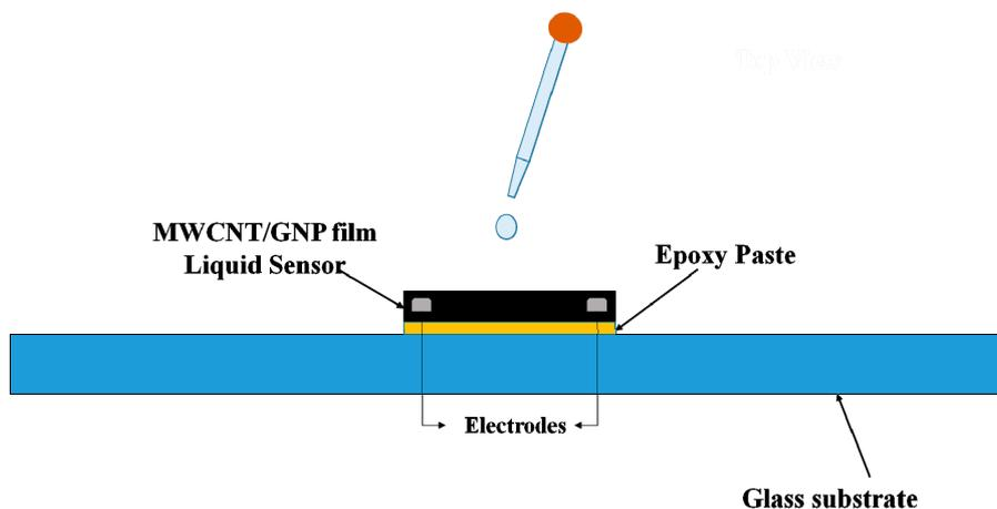
Figure 14. Schematic diagram of the titration test on the hybrid film.
