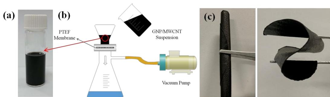
**Figure 2.** (a) MWCNT/GNP hybrid suspension, (b) schematic diagram of vacuum filtration, and (c) a flexible GNP/MWCNT hybrid film.
