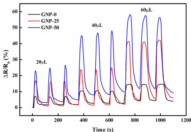
**Figure 17.** Resistance changes of the hybrid films in consecutive cycles of infiltration and evaporation of acetone drops.
