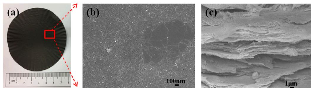
**Figure 5.** GNP-50 film with 50 wt% graphene and 50 wt% MWCNT; (a) the prepared film, (b) surface morphology SEM image, and (c) cross-section SEM image.
