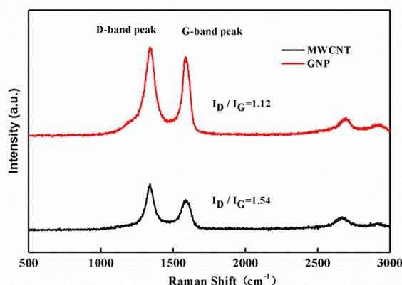
**Figure 1.** Raman spectrum of the graphene nanoplatelets (GNPs) and the multi-walled carbon nanotubes (MWCNTs).
