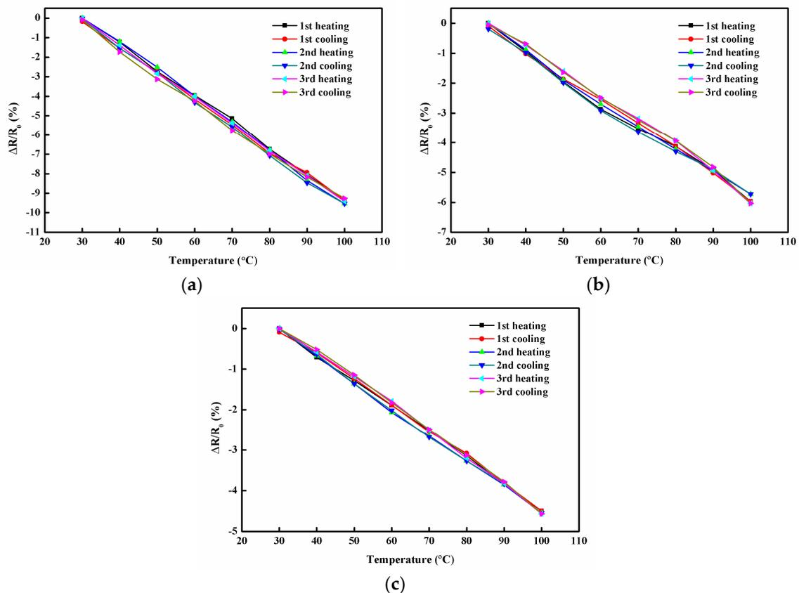
**Figure 12.** Normalized relative resistance change of the hybrid films subjected to cyclic heating and cooling tests. (a) GNP-0 with 0 wt% GNP and 100 wt% MWCNT. (b) GNP-25 with 25 wt% GNP and 75 wt% MWCNT. (c) GNP-50 with 50 wt% GNP and 50 wt% MWCNT.
