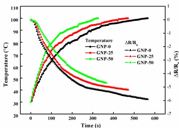
**Figure 13.** Temperature and resistance responses of the hybrid films placed in an oven at temperature of 100 °C.
