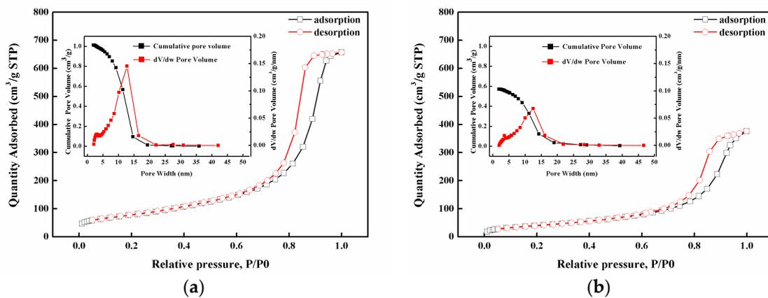
**Figure 8.**  $N_2$  adsorption–desorption isotherms. Insets show the BJH pore size distribution. (a) GNP-0 with 0 wt% GNP and 100 wt% MWCNT and (b) GNP-50 with 50 wt% GNP and 50 wt% MWCNT.
