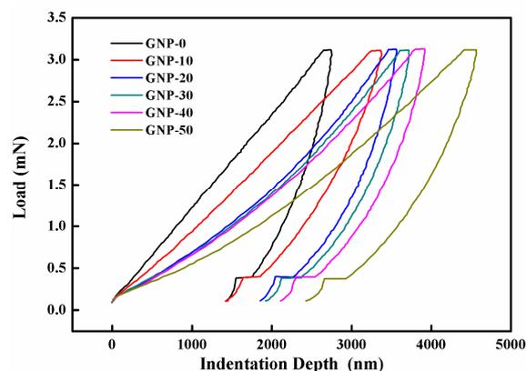
**Figure 9.** Load versus indentation depth curves for the hybrid films with different weight percentages of GNP.
