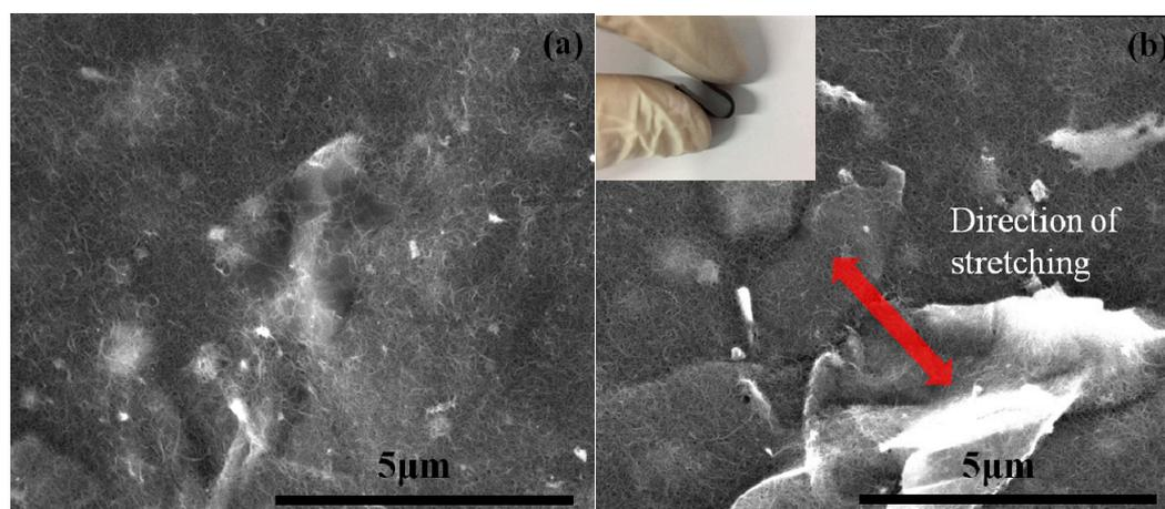
**Figure 3.** SEM images of the hybrid film GNP-50, (a) before and (b) after bending.
