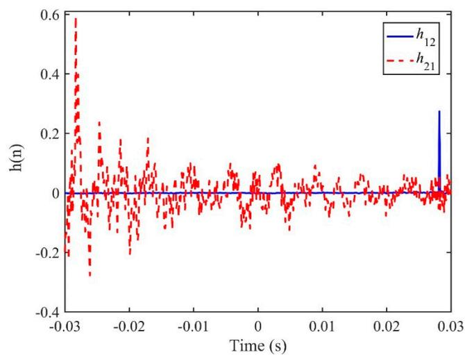
**Figure 14.** IRFs between the signals measured at A2&A3 using the conventional LMS adaptive method.
