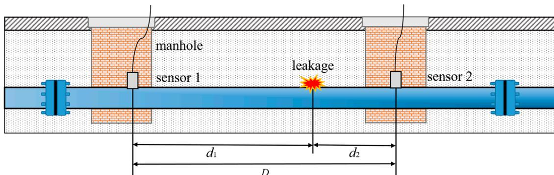
Figure 1. Schematic of leak detection measurements in water distribution pipes.
