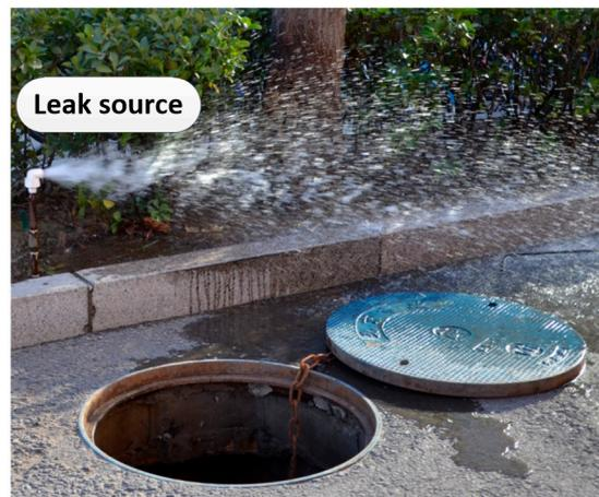
**Figure 11.** Leak generated above the ground.
