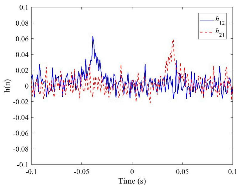
Figure 5. IRFs given by the conventional LMS adaptive method.
