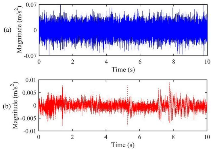
**Figure 12.** Leak signals measured by the accelerometer pair of (a) A2; (b) A3.
