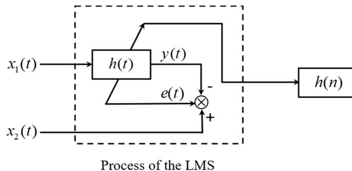
**Figure A1.** Schematic of the implementation of the LMS adaptive method.
