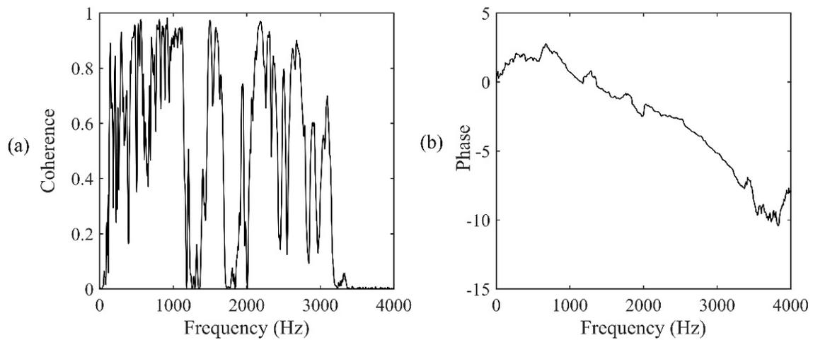
**Figure 18.** Frequency analysis of the signals measured at A1&A3: (a) Coherence function; (b) phase spectrum.
