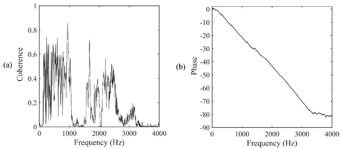
**Figure 13.** Frequency analysis of the signals measured at A2&A3: (a) Coherence function; (b) phase spectrum.
