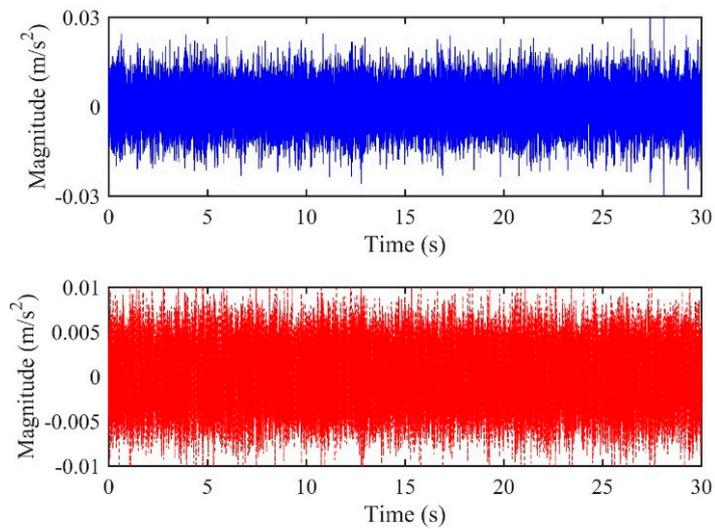
**Figure 17.** Leak signals measured by the accelerometer pair of (a) A1; (b) A3.
