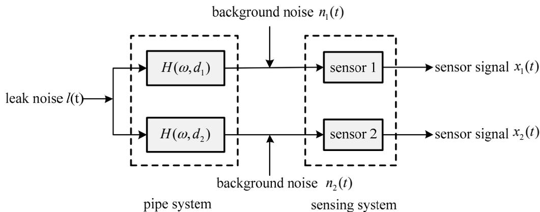
Figure 2. Flow diagram of leak noise measured by two sensors.
