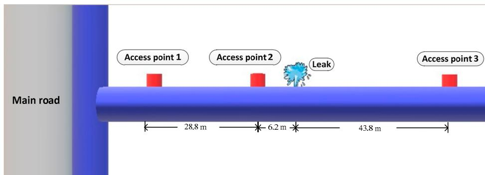
**Figure 9.** Schematic of the test site located at the IACAS.
