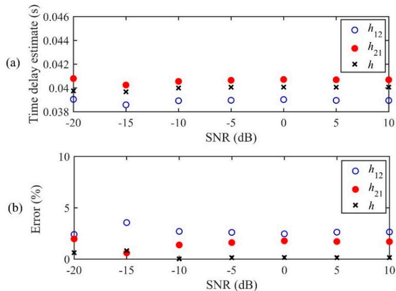
**Figure 8.** Effect of background noise on the performance of the adaptive methods for TDE: (a) Time delay estimate; (b) relative error.
