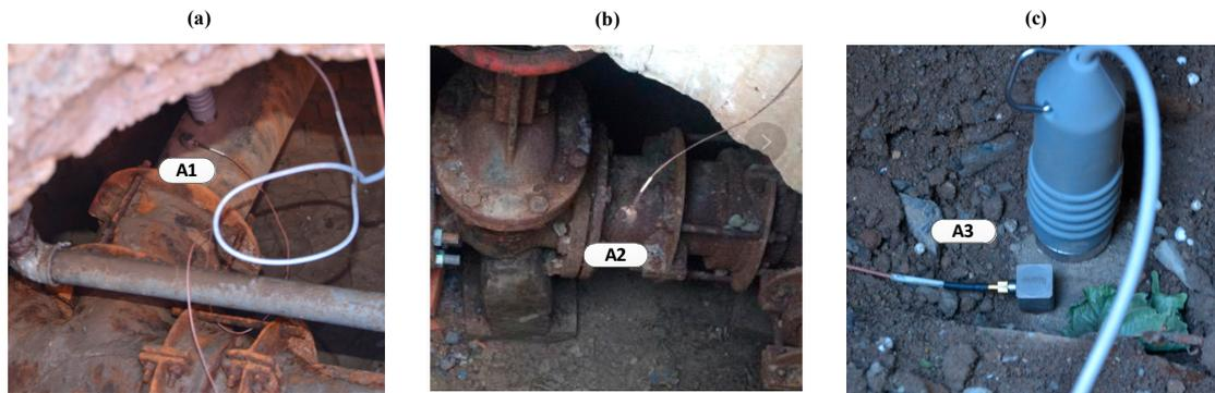
**Figure 10.** Accelerometers attached magnetically to the test pipe. (a) At access point 1; (b) At access point 2; (c) At access point 3.
