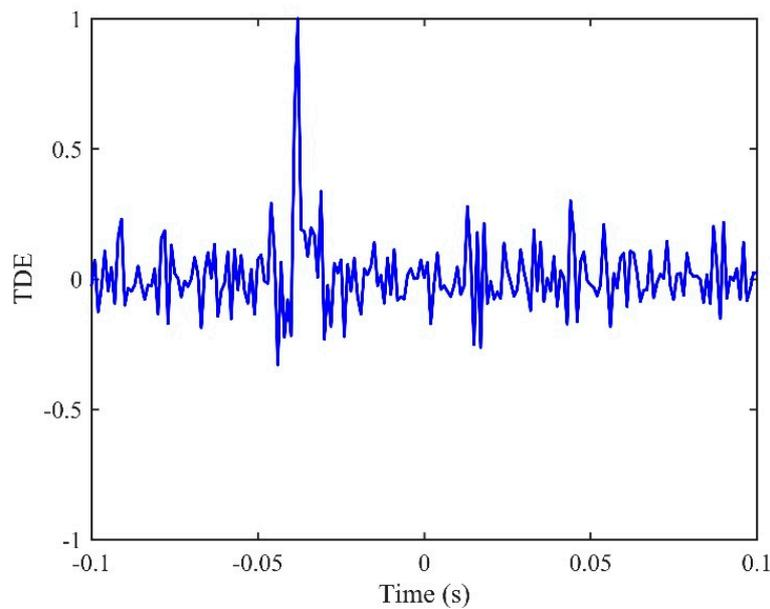
Figure 7. The IRF given by the proposed ADPHAT method for TDE.
