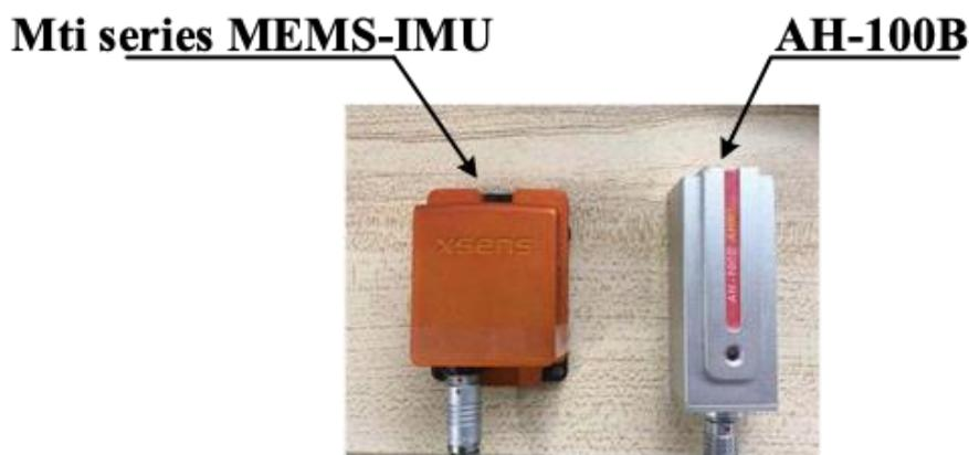
**Figure 14.** Experiment apparatus, Mti series MEMS-IMU from Xsens and AH-100B.
