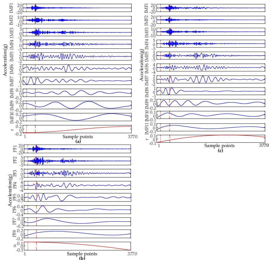
Figure 4. The time domain segmentation of EMD, LMD, and EEMD: (a) IMFs decomposed by EMD method; (b) PFs decomposed by the LMD method; (c) IMFs decomposed by the EEMD method.
