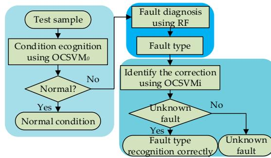
Figure 1. Diagnosis process of the hybrid classifier.
