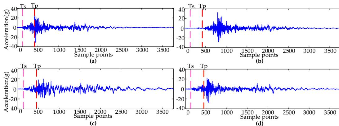
**Figure 3.** Measured vibration signals and the time domain segmentation unit: (a) The normal condition; (b) The iron core stagnation; (c) The screw loosening condition; (d) The poor lubrication condition.
