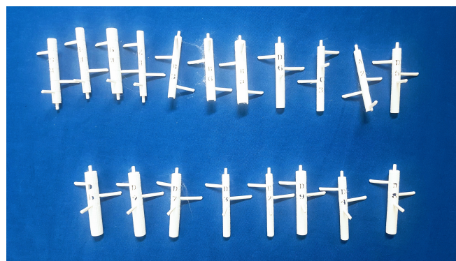
Figure 9. Marker tools. We used an inexpensive 3D printer to create marker tools with various sizes and patterns.
