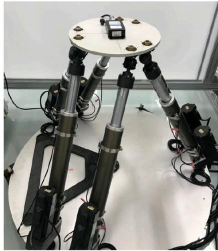
**Figure 6.** The Stewart platform for the MEMS inclinometer testing.
