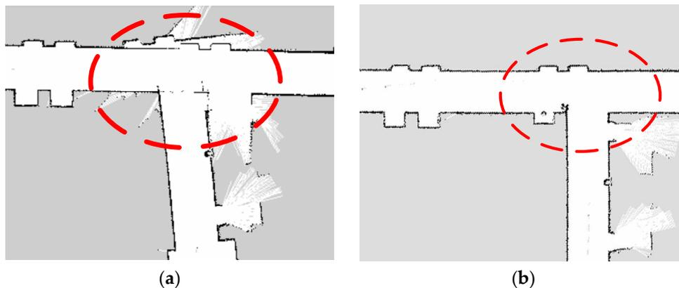
**Figure 13.** Ring corridor closed-loop connection for map construction before (a) and after (b) the calibration.
