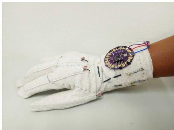
**Figure 4.** Side view of the wireless smart glove. No external power or wired data transmission are required.
