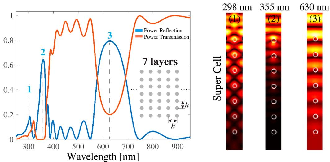
**Figure 4.** (left) Spectral response of the power reflection/transmission for the same configuration in Figure 1, but for seven layers along the  $y$ -axis. (right) Near field  $|H_z|$  distributions at three different peak wavelengths, i.e. 298 nm (associated with the Rayleigh wavelength), 355 nm (associated with a resonance wavelength of a single silver nanocylinder), and 630 nm (associated with plasmonic gap in Figure 1).
