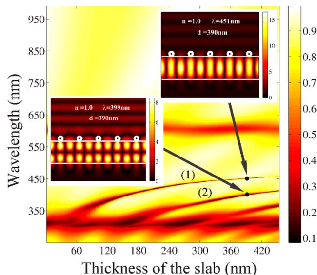
**Figure 7.** Plasmonic grating as refractive index sensor: Contour plots of transmission spectra versus thickness of the slab  $d$  at  $n = 1$ . Simulated near field distributions of  $|H_z|$  at  $\lambda = 451$  nm and  $\lambda = 399$  nm for a fixed thickness of the slab  $d = 390$  nm are shown as insets.
