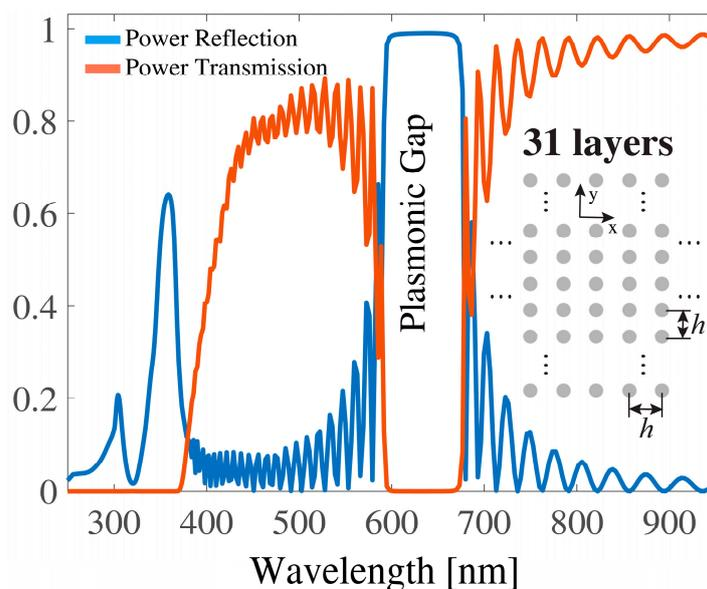
**Figure 1.** Power reflection (blue line) and power transmission (red line) of a 31-layered plasmonic crystal formed by the corresponding periodical arrangement of cylindrical Ag nanocylinders. Period of the grating was equal to  $h = 300$  nm and radius of the nanocylinder amounts to  $r = 40$  nm. Excitation was provided by an impinging H-polarized plane wave ( $H_z, E_x, E_y$ ) with normal incidence (along the positive  $y$ -axis).
