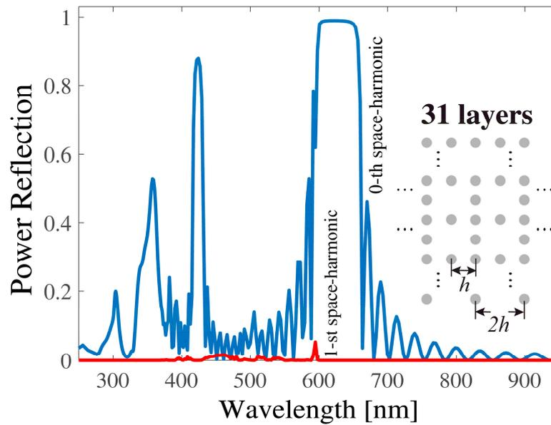
**Figure 3.** The same settings as in Figure 1, but the crystal was formed by alternately stacking the complete layer with a period  $h$  and the defect layer, where one nanocylinder was periodically removed according to the period  $2h$ .
