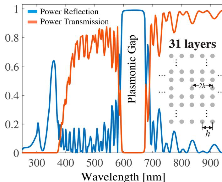
**Figure 2.** The same settings as in Figure 1, except that the intermediate 16th layer of the original crystal was replaced by a defect layer where one nanocylinder was periodically removed with a period of  $2h$ .
