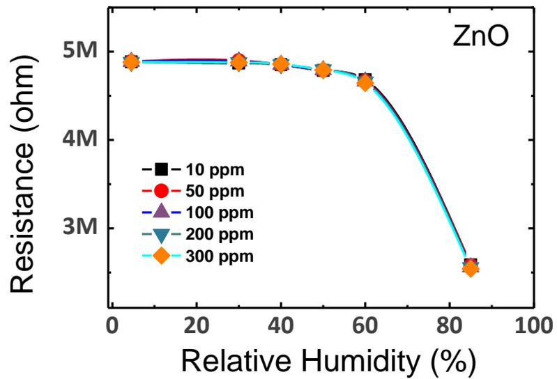
Figure S5. Response of ZnO thin film to varying NH<sub>3</sub> concentration and relative humidity.
