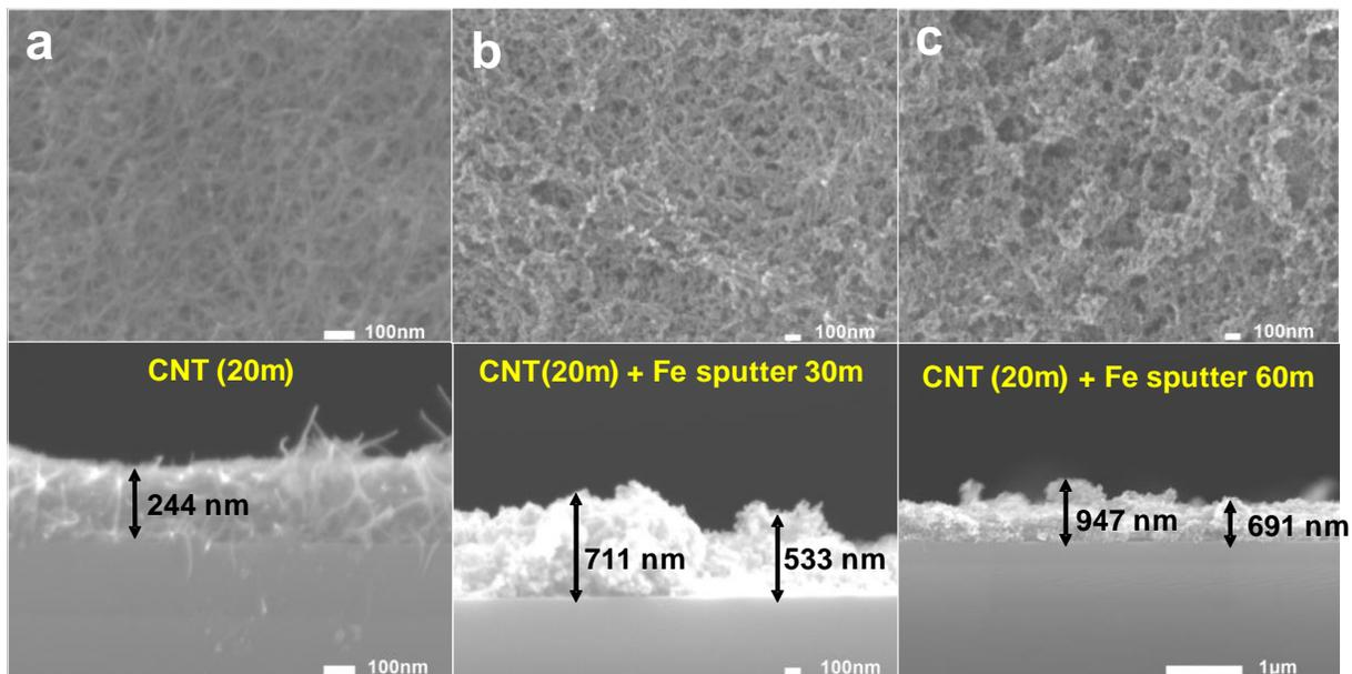
**Figure S3.** (a) SEM images of the SWCNT mat fabricated by the arc-discharge for 20 min followed by the methanol treatment. (b) Hematite ( $\text{Fe}_2\text{O}_3$ ):CNT composite structures fabricated by the sputter deposition of Fe on the SWCNT mat for 30 min and (c) 60 min followed by oxidation at 400 °C for 2 h.
