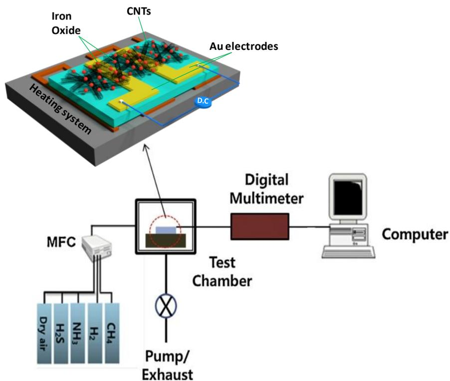
**Figure S2.** Schematic diagram of the sensor measurement system with the magnified sensor device configuration.[1].
