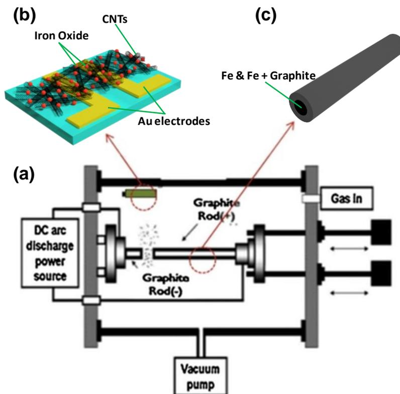
**Figure S1.** (a) Schematic diagram of the arc-discharge system. (b) The schematic sensor device structure deposited with single-wall carbon nanotubes (SWCNTs) dispersed with iron oxides on Au-electrode patterned alumina substrate. The substrate was mounted on the inside wall of the chamber for the iron (Fe):CNT composite deposition. (c) The graphite tube used as the arc-discharging source. The hollow tube was filled by the controlled mixture of Fe and graphite powder. [1].
