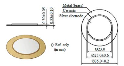
Figure 1. Murata piezoelectric sensor 7BB-35-3 used in the tests.
