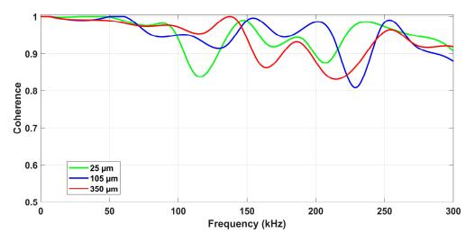
**Figure 6.** Magnitude-squared coherence between the AE sensor and PZT diaphragm at three grinding conditions.
