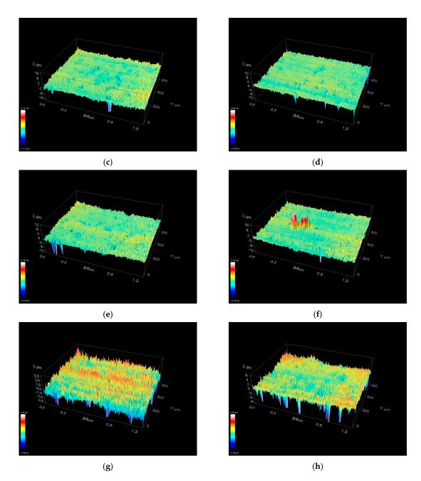
**Figure 3.** Confocal microscopy: (**a**) Without cutting; (**b**) 25 μm; (**c**) 35 μm; (**d**) 50 μm; (**e**) 105 μm; (**f**) 150 μm; (**g**) 210 μm; and (**h**) 350 μm.
