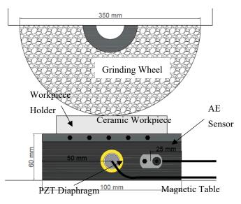
Figure 2. Experimental setup.
