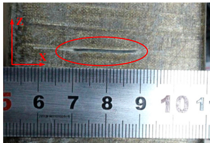
Figure 10. The surface crack damage.
