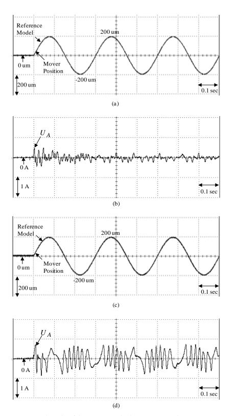
**Figure 10.** Experimental results of the micrometer backstepping control system using an amended recurrent Gottlieb polynomials neural network and AACO with the compensated controller for the periodic sinusoid command: (**a**) mover position in the rated case; (**b**) control intensity in the rated case; (**c**) mover position in the parametric variation case; (**d**) control intensity in the parametric variation case.
