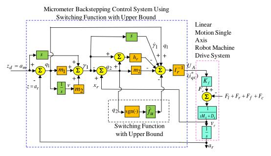
Figure 6. Micrometer backstepping control system using switching function with upper bound.
