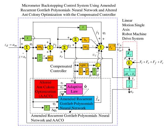
**Figure 3.** Micrometer backstepping control system using an amended recurrent Gottlieb polynomials neural network and altered ant colony optimization with the compensated controller.
