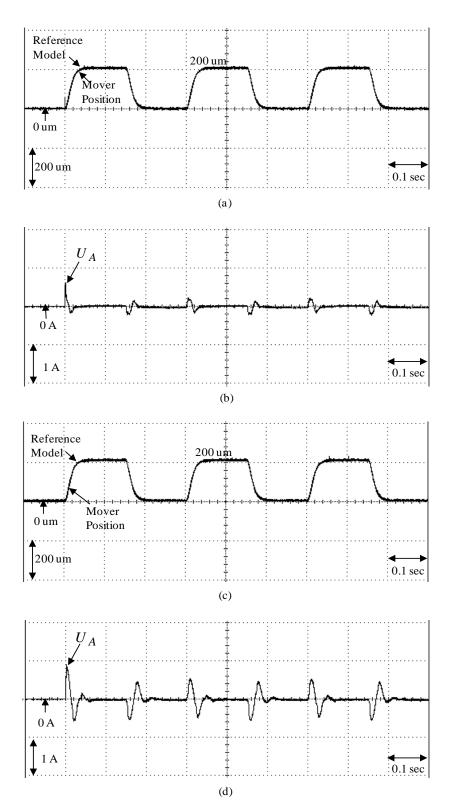
**Figure 9.** Experimental results of the micrometer backstepping control system using an amended recurrent Gottlieb polynomials neural network and altered ant colony optimization (AACO) with the compensated controller for the periodic step command: (**a**) mover position in the rated case; (**b**) control intensity in the rated case; (**c**) mover position in the parametric variation case; (**d**) control intensity in the parametric variation case.
