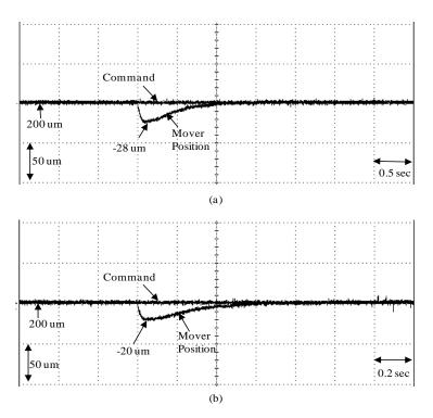
**Figure 11.** Experimental results of measured mover position response under the step force disturbance with adding load  $f_L = 2N$  in the 200um: (a) for the micrometer backstepping control system using switching function with upper bound; (b) for the micrometer backstepping control system using an amended recurrent Gottlieb polynomials neural network and AACO with the compensated controller.
