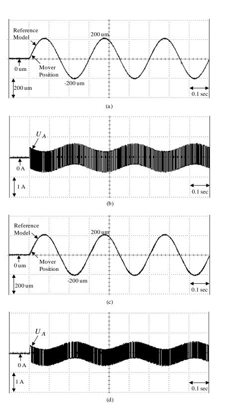
**Figure 8.** Experimental results of the micrometer backstepping control system using the switching function with an upper bound for the periodic sinusoid command: (**a**) mover position in the rated case; (**b**) control intensity in the rated case; (**c**) mover position in the parametric variation case; (**d**) control intensity in the parametric variation case.
