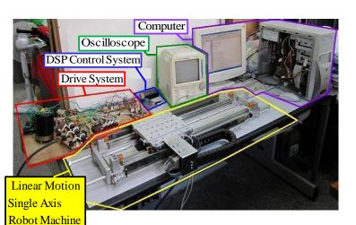
Figure 5. A picture of the experimental set-up of the linear motion single axis robot machine drive system.
