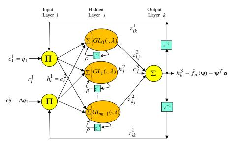
Figure 4. Makeup of the three-layer amended recurrent Gottlieb polynomials neural network.
