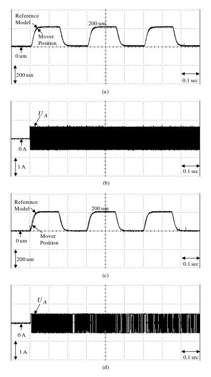
**Figure 7.** Experimental results of the micrometer backstepping control system using the switching function with an upper bound for the periodic step command: (**a**) mover position in the rated case; (**b**) control intensity in the rated case; (**c**) mover position in the parametric variation case; (**d**) control intensity in the parametric variation case.
