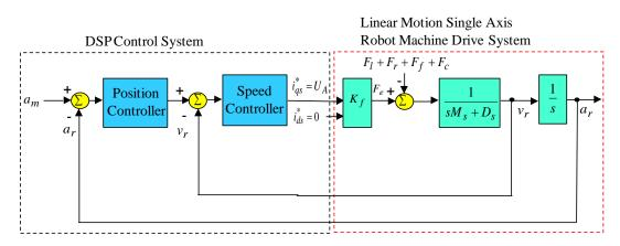
Figure 2. Simplified block diagram of linear motion single axis robot machine drive system.
