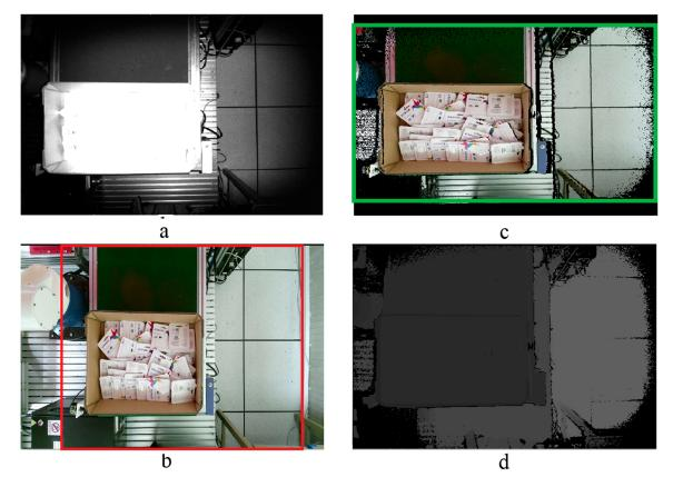
**Figure 10.** (a) IR image, (b) original image, (c) registered color image and IR obtained from transformation and cropping, (d) depth image.
