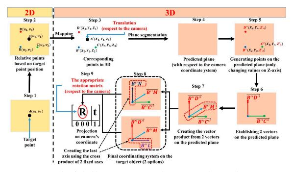
**Figure 15.** Procedure for building an appropriate coordinate system on the target object to create a rotation matrix with respect to the camera.
