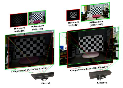
**Figure 9.** Kinect v1 and v2 overlap regions in the captured scene. The green rectangle represents the RGB view, and the red rectangle represents the IR view [47].
