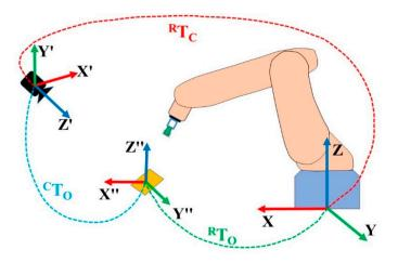
Figure 16. Camera and object position with respect to the robot base.
