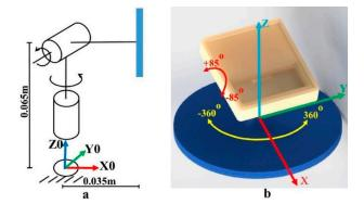
**Figure 17.** (**a**) Kinematic model, (**b**) a supportive platform to capture the object's ground truth with respect to the robot (for both the front and back sides).
