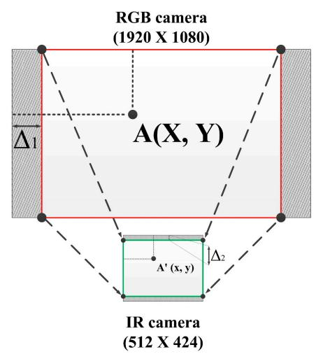
Figure 11. Demonstration of mapping methodology for Kinect v2.
