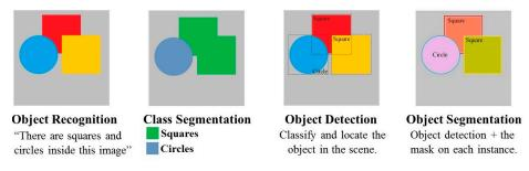
Figure 5. Typical image processing task.
