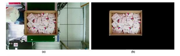
**Figure 22.** Image preprocessing to remove unnecessary information—(**a**) the original RGB image captured by the camera; (**b**) the result after removing the unnecessary information.
