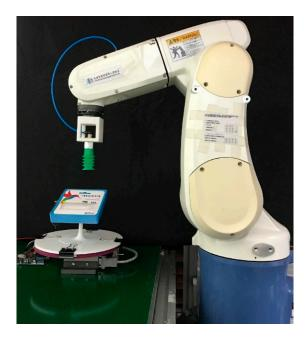
Figure 28. Support platform to take the ground truth of objects in the working area.
