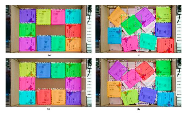
Figure 19. (a,c) Ground truth of two test cases; (b,d) the results of the prediction corresponded to two ground truths.
