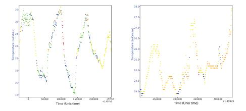
**Figure 5.** The temperatures for two different days and the correlation with the wind direction. The direction of the wind is represented by the different dot colors with blue to be a North–South direction and with red a West–East direction. On the left we have a couple of days at the middle of the measurement period and on the right a couple of days at the end of the measurement period.
