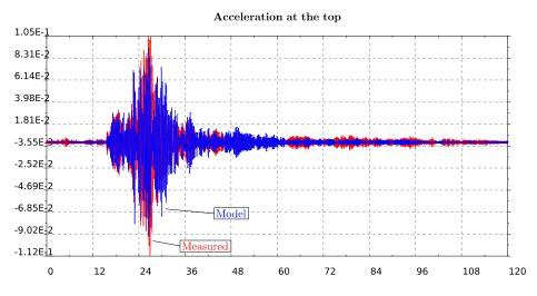
**Figure 13.** Response of top level acceleration for the East–West model (top plot) and for the North–South (bottom plot), respectively. Both recorded motion (red) and computed by the model (blue) are presented.
