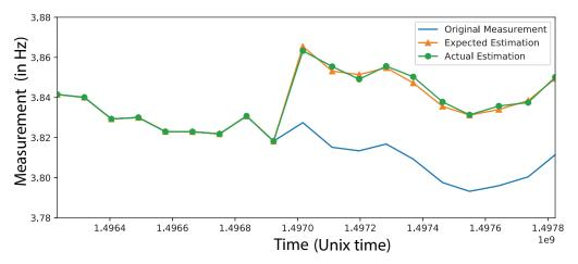
**Figure 8.** The estimation of first mode using a 24-hour time window for the current quantity and imposing shift of 1%. With orange we plot the exact imposed shift and with green we plot the estimation provided by the SM. We observe very good agreement.
