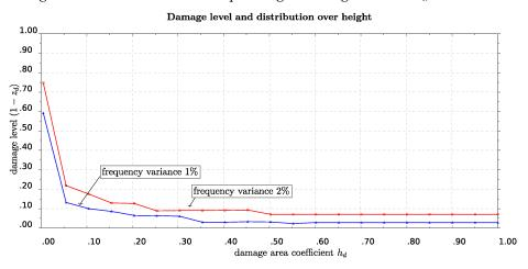
**Figure 11.** Combination of damage level *z* with damaged area length  $h_d L$ , for variation of eigenfrequency  $\Delta v = 1\%$  and 2%.
