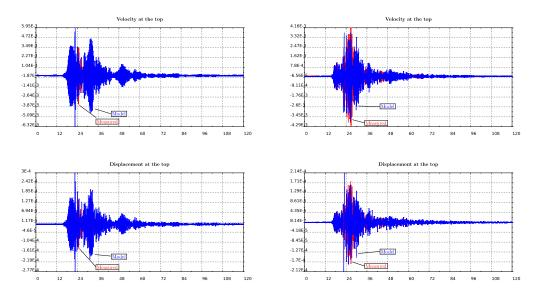
**Figure 14.** Response of top level velocities (top) and displacements (below) for the East–West model (left) and for the North–South (right), respectively. Both recorded motion (red) and computed by the model (blue) are presented.
