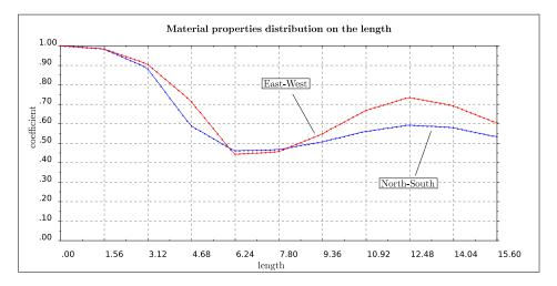
**Figure 10.** Material properties (elasticity modulus, mass density) nondimensional distribution (vertical axis) with the height (horizontal axis) of the lighthouse.
