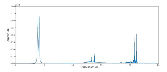
**Figure 3.** The first singular value of the reference cross-correlation matrix (computed using the first 8 days of acquisition) as a function of frequency (in Hz),  $\sigma_1^r(\nu)$ . The estimated values for the first seven natural frequencies of the structure are given in Table 1.
