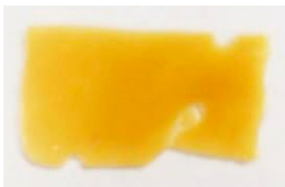
Figure S3 Urea sensing hydrogel which contains microcapsules with BSA-modified MPy-AgNP cargo and urease conjugated to the matrix. The yellow color results from the BSA-modified MPy-AgNPs.
