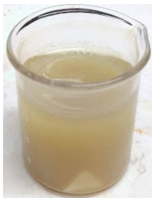
Figure S2 \text{CaCO}_3 microspheres containing BSA-modified MPy-AgNPs. In absence of BSA (microspheres containing MPy-AgNPs) a dark gray color results instead of the yellow-gray color seen above.
