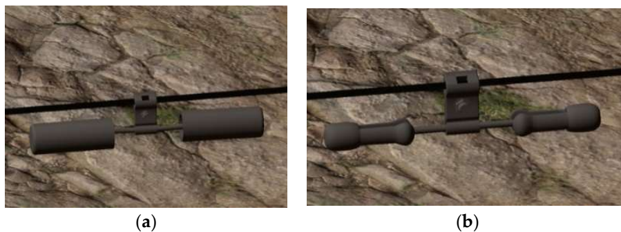
Figure 6. The two types of vibration-dampers. (a) FD type; (b) FR type.
